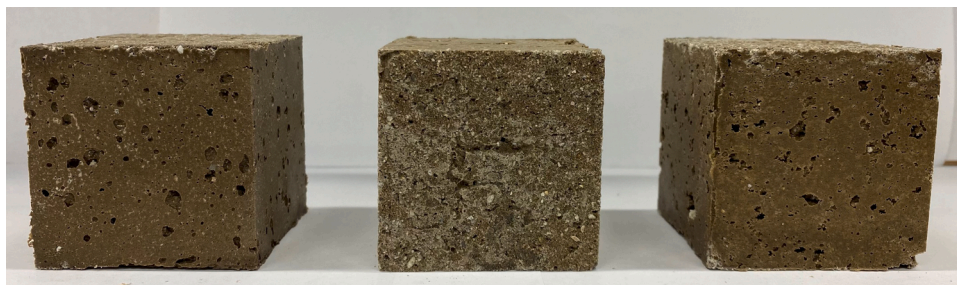
Fig. 2. Encapsulation of rPU previously pre-impregnated with kerosene + 30%v. TBP in cubic geopolymer samples (side of 5 cm). From left to right, the rPU polymer loading factor is 5, 10, and 10%wt., the kerosene + 30%v. TBP loading factor is 10, 10, and 20%wt.
