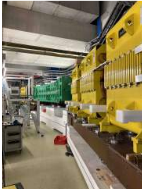
Figure 2.5: Magnetic elements in the FRS: a dipole (green) and a series of quadrupoles (yellow) before and after.
