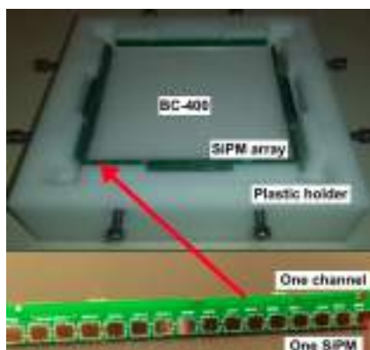
Figure 2.18: Picture of a \beta Plastic detector out of the beamline. The scintillator material and the SiPM readout are highlighted by labels.
