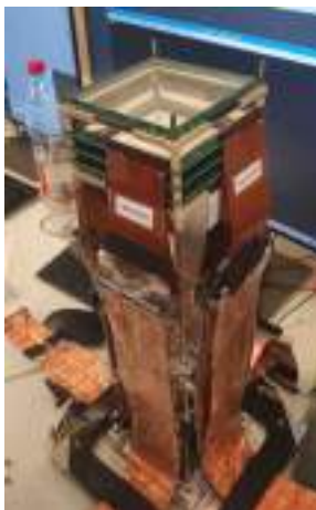
Figure 2.17: Picture of the AIDA detectors on the test bench. The three DSSD layers are sandwiched between the two \beta plastic detectors.
