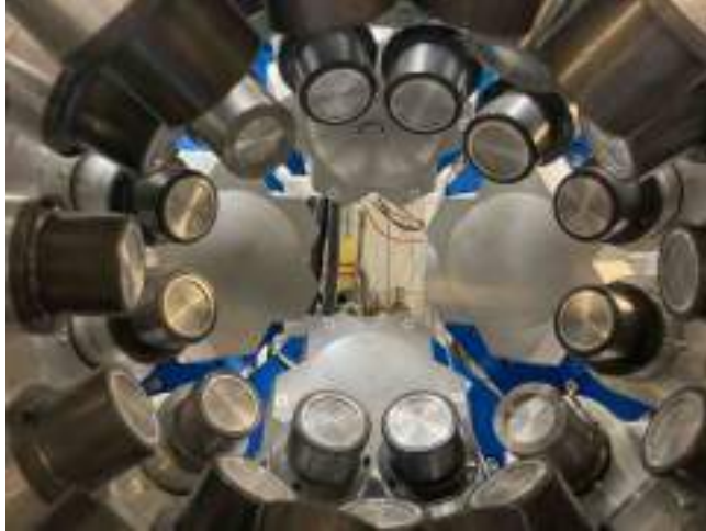
Figure 2.20: Picture of a the euroball array from the upstream point of view. The clusters are positioned in a cross configuration in forward position, after the FATIMA array.
