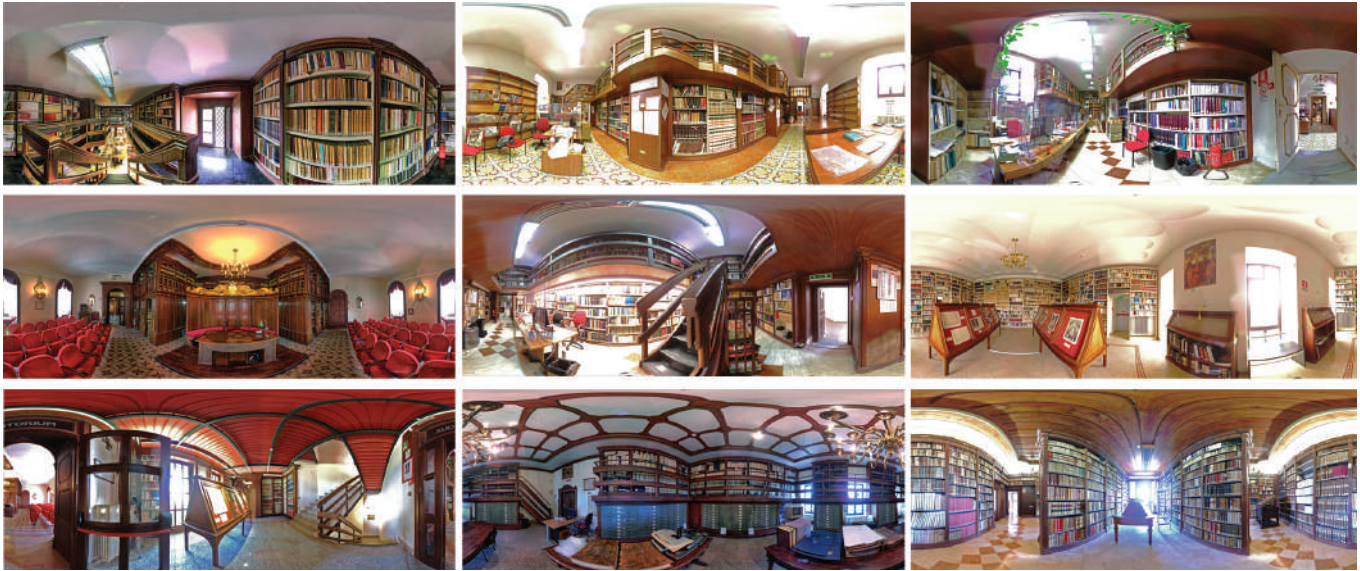
Figure 3. Some of the panoramic images of the Loreto di Montevergine Abbey Palace, in equirectangular projection, captured by the laser scanner camera.
