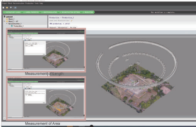
Figure 7. Measurement of site height, area and earthwork volume.
