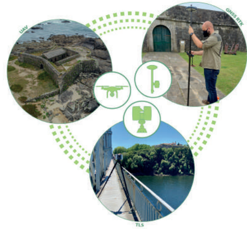
Figure 3. The technologies applied for the integrated survey.
