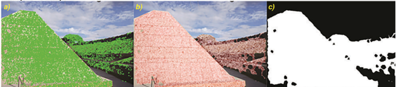
Figure 3. a): Identification on the image of the TP inside the confidence interval (green pixels); b): Alpha Shape triangulation (transparent red); c): Binary mask.
