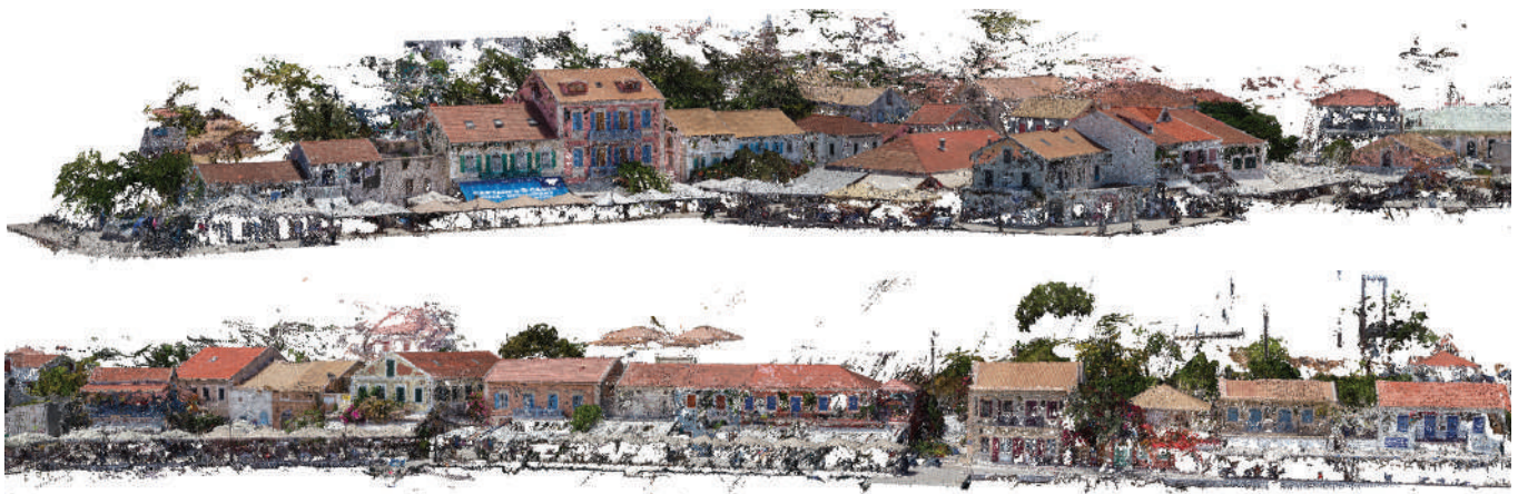
Figure 7-8. Port of Fiskardo, dense cloud, southern view - Port of Fiskardo, dense cloud, northern view.
