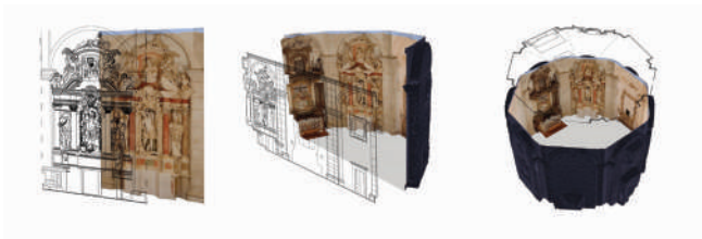
Figure 11. Overlap between the models obtained by SfM and the 2D drawings that have been obtained, relating to the altar of St. Michael, the cross section and the plan. The elaboration is by Luca Cetra.
