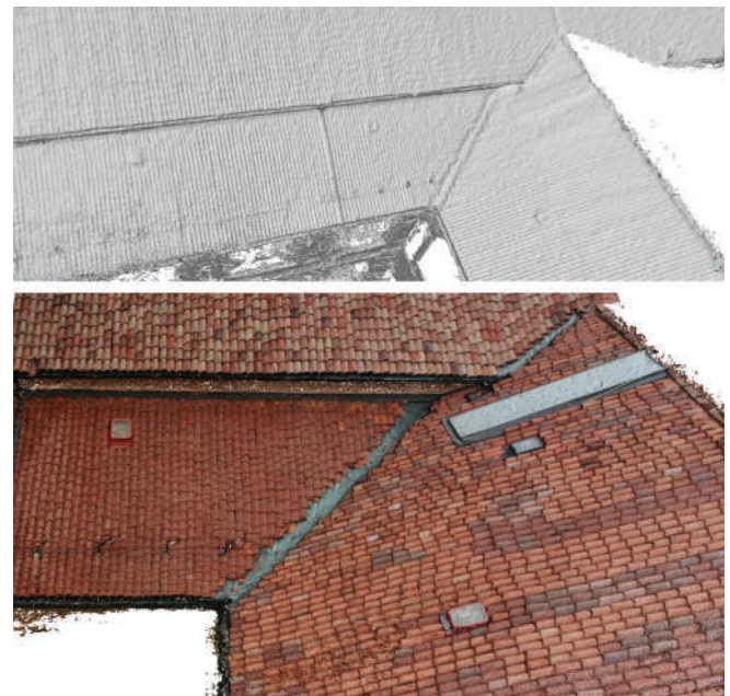
Figure 5. Dense point cloud elaborated with SfM process from Ultra-Light UAV (DJI Spark) survey.
