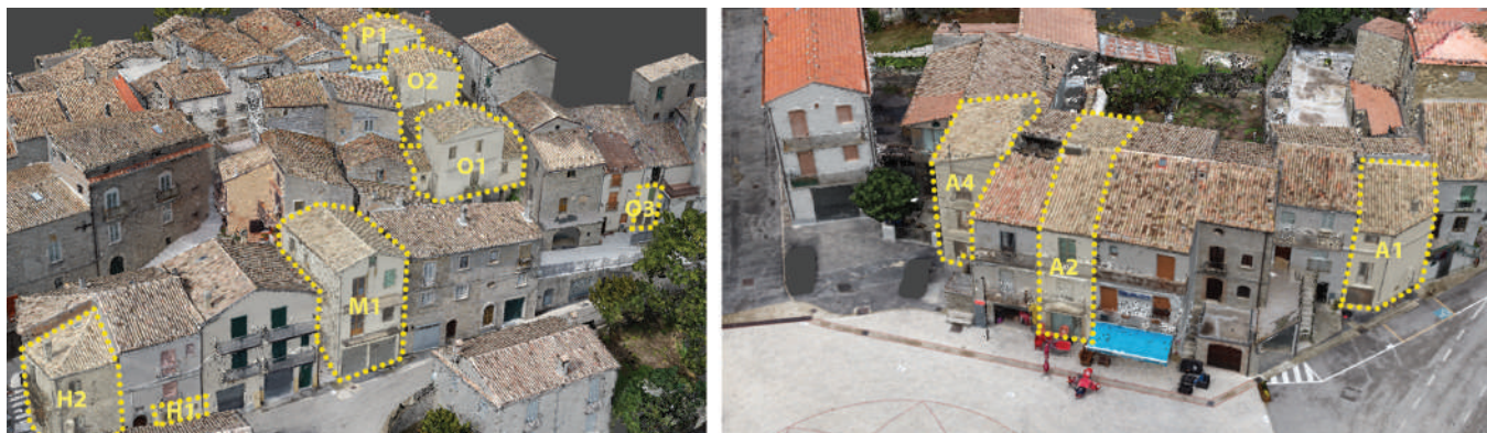
Figure 4. Mesh models of the historic centre. The analysed building units are highlighted and indicated with an alpha-numerical code in which the letter specifies the aggregate while the number defines units studied inside. (Source: Authors' graphic elaboration).
