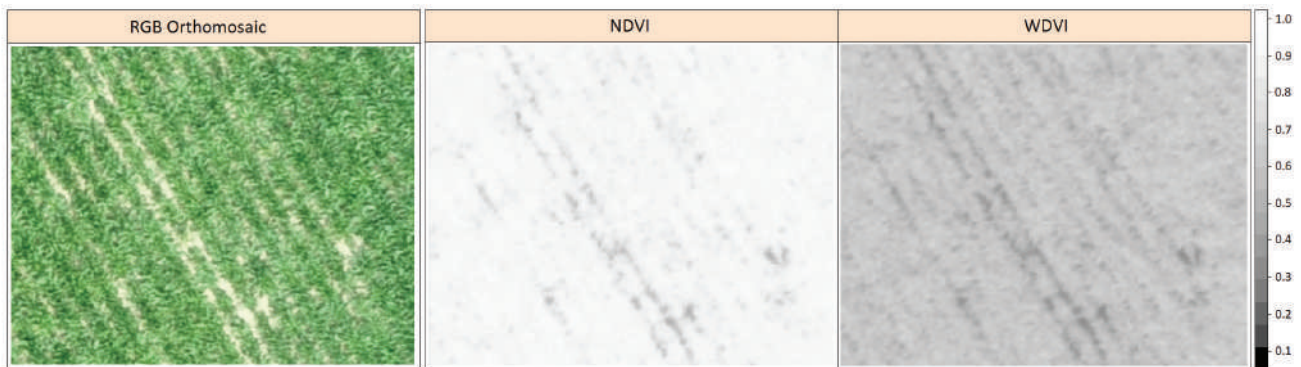
Figure 2. On the Cover: True color composite RGB orthomosaic over an area of the study field where the soil background is visible (left) along with the corresponding NDVI (middle) in which the index is highly saturated, while WDWI (right) exhibits a sharper soil background that enables proper discrimination between vegetation and soil clusters.
