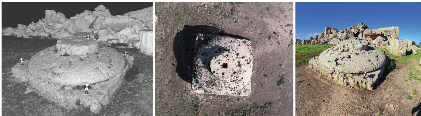
Figure 11 Capital at the SE corner of the Temple: laser scanning (left) and photogrammetric survey from photos taken by the UAV (middle) and the action camera (right).
