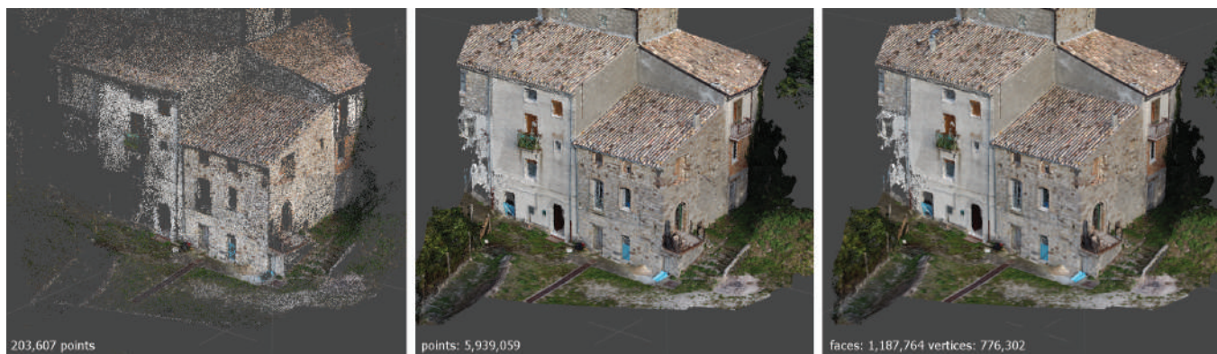
Figure 6. Processing of Unit N1, from left to right: Sparse point cloud; Dense point cloud; 3D mesh model. (Source: Authors' graphic elaboration).
