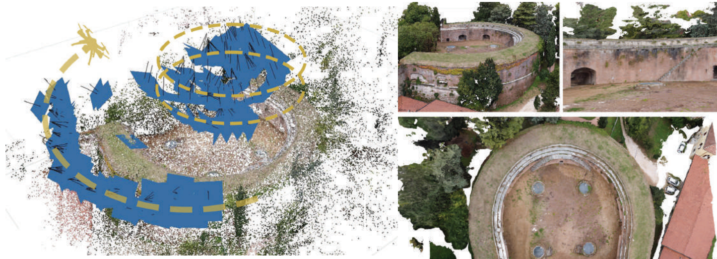
Figure 8. Scheme acquisition with UAV through the use of DJI Mavic Mini 2 drone of the open-air shooting platform that characterizes the bastion. At right, a collection of images of the 3D model generated from the point cloud alignment, using the software Agisoft Metashape.
