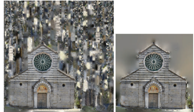
Figure 5. S. Salvatore dei Fieschi Church, Cogorno. Differences between texture types. Left: an adaptive orthophoto. Right: a simple orthophoto. (Postgraduate School thesis; students: Luca Formigari, Davide Felici).
