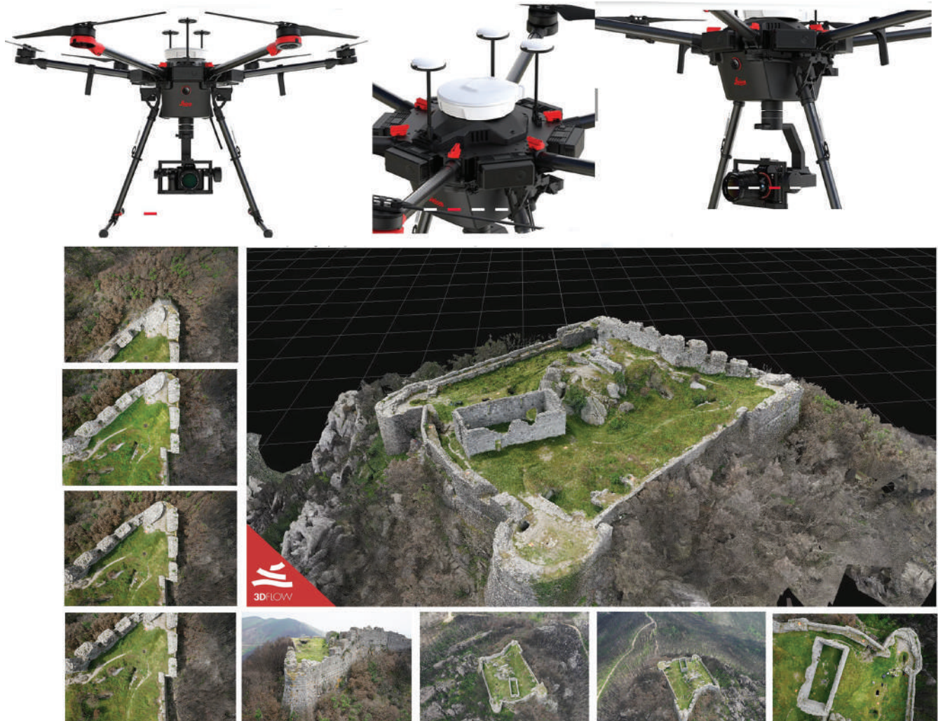
Figure 3. Image based and UAV survey methodologies, used for the reconstruction of the fortress.
