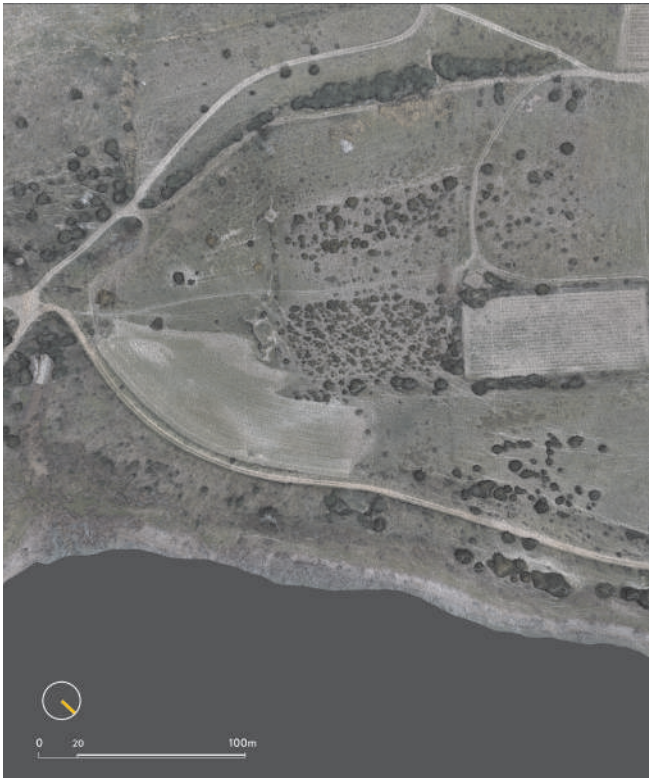
Figure 2. Survey area (orthophoto generated by point cloud with 0,025 m/pix of GSD).
