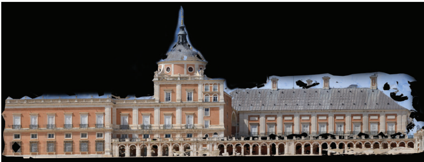
Figure 5. Royal Palace of Aranjuez, southward view of the side elevation, precision orthophoto from textured mesh. (Gennaro Pio Lento, 2022)
