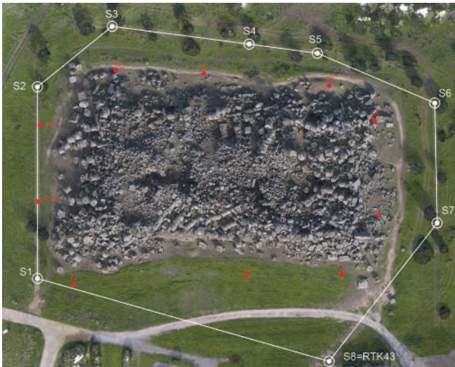
Figure 4. Top view of the point cloud, the topographic polygonal (white) and the rectangular markers (red).
