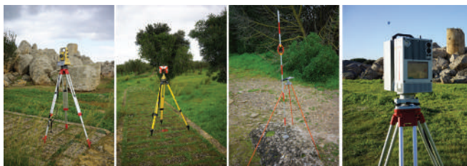
Figure 2. Topographic and laser scanning surveying sessions.
