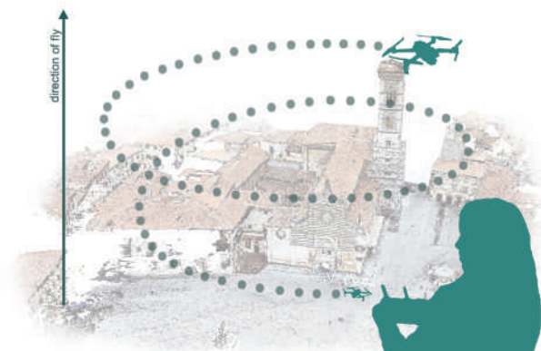
Figure 6. Spiral acquisition scheme of the Prato Cathedral complex and square with DJI Mavic 2.
