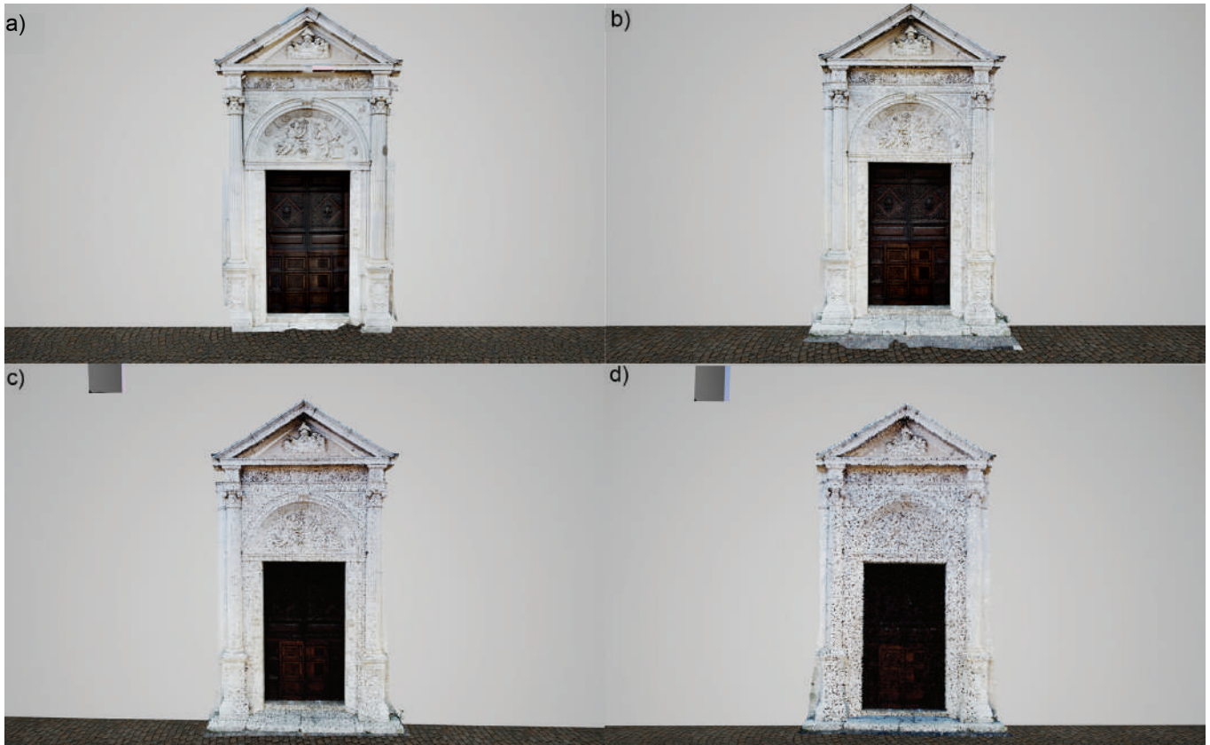
Figure 8. Virtual model of the Church’s portal based on the four dense point clouds.
