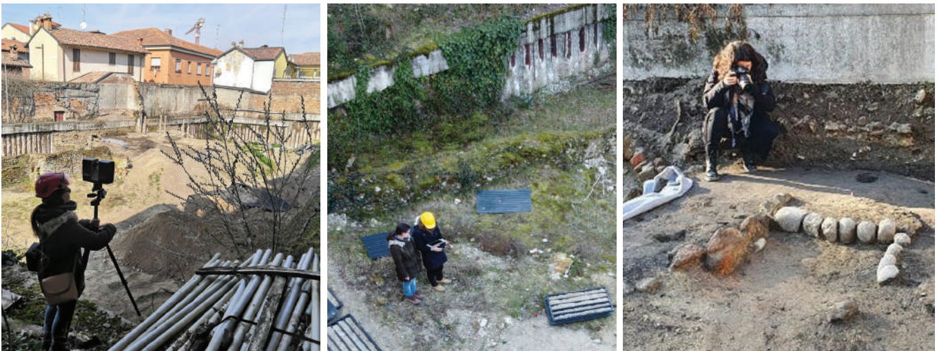
Figure 5. From left to right: Extensive survey with CAM2 Laser scanner FOCUS; Broad survey with DJI MAVIC MINI 2; Detailed survey using Canon EOS 70D.
