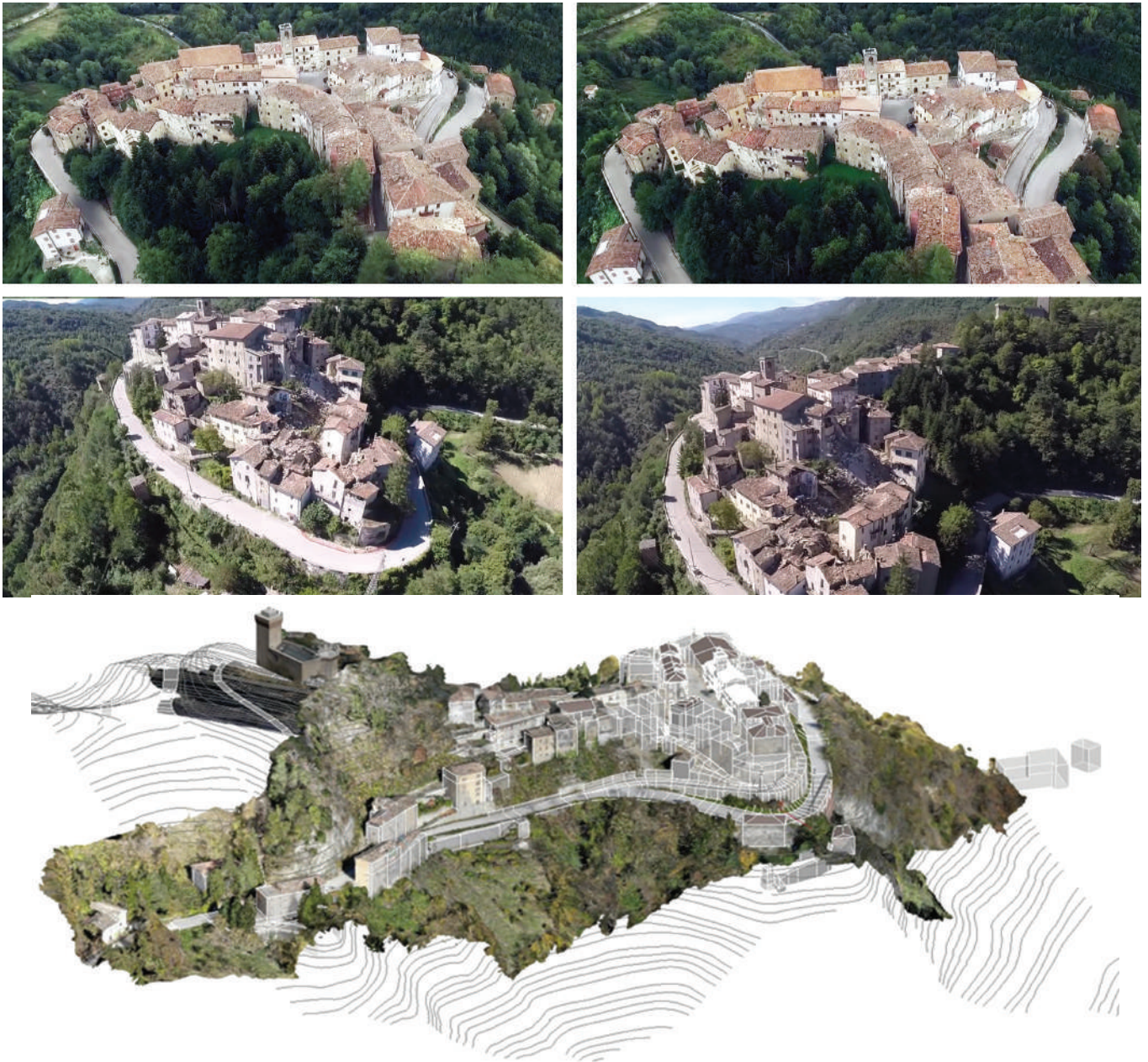
Figure 6. Above, 2 frames of a pre-seismic flight (July 2016) and 2 frames of a flight after the first seismic shock (August 2016) (by M. Canciani). Below, volumetric model of the pre-seismic situation (August 2016). (by M. D'Angelico)
