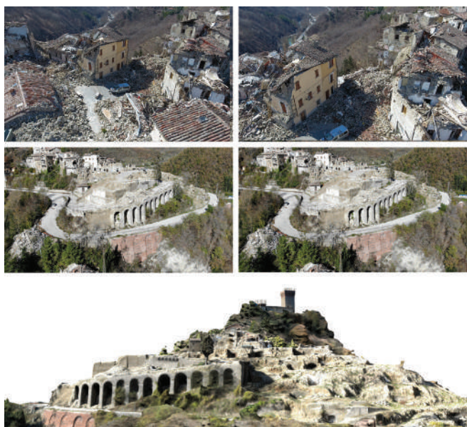
Figure 7. Above, 2 frames of a second-seismic shock (November 2016) and 2 frames of a flight after the debris removal (April 2018) (by M. Canciani). Below, volumetric model of the post-seismic situation (April 2018). (by M. D'Angelico)
