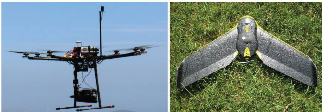
Figure 1. Mainly used UAV: octocopter with a light detection and ranging (LiDAR) sensor (left) and fixed-wing eBee drone (right).
