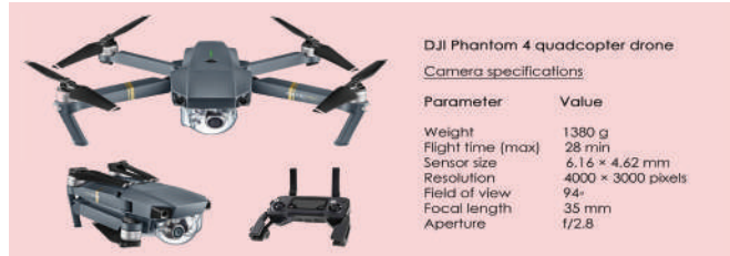
Figure 5. DJI Phantom 4 quadcopter drone - camera specifications.
