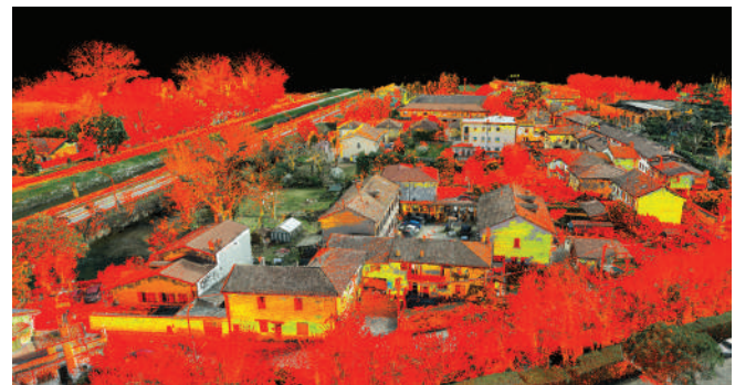
Figure 8. View of merged point clouds. The image shows the necessity to use UAV acquisition to complete the datas of the inner areas.
