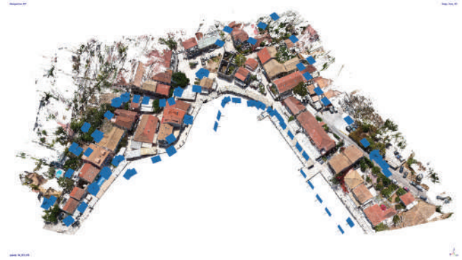
Figure 5. Port of Fiskado, dense cloud with cameras, top view.
