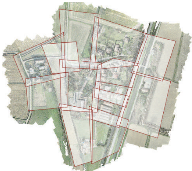
Figure 5. UAV's acquisition plan on Cassinino settlements, with the division in 13 sub-areas.
