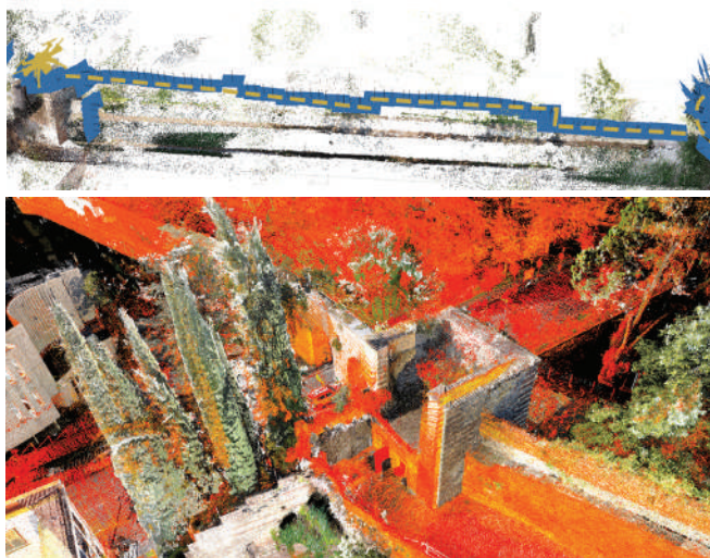
Figure 9. Scheme acquisition with UAV through the use of DJI Mavic Mini 2 drone of the tower. The drone data was subsequently processed through optimization operations of the point cloud and alignment of the data acquired by laser scanner. This operation made it possible to have an integrated and stratified 3D point cloud database.
