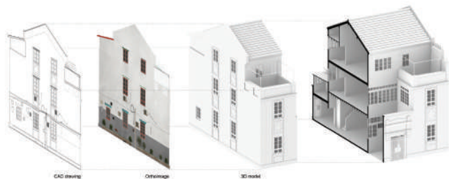
Figure 10. Survey results example: CAD drawing, orthophoto and 3D model (software: Rhinoceros).
