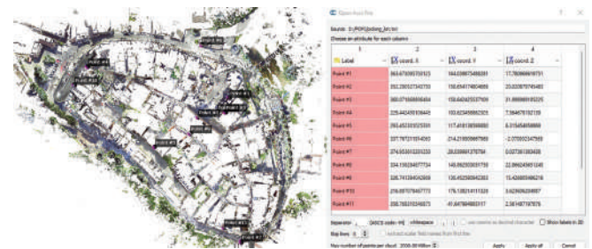
Figure 7. Query of structured point cloud and coordinates acquisition.
