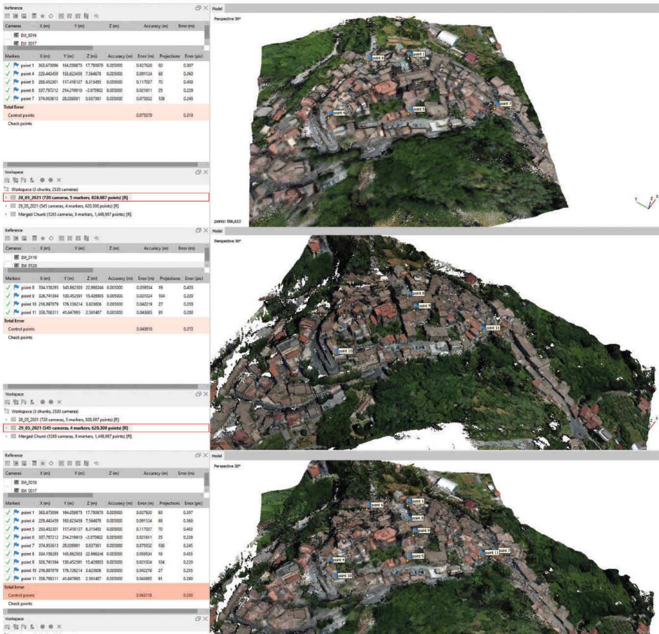
Figure 8. Creation of dense clouds scaled based on coordinates from TLS and automatic integration of the two numerical models.
