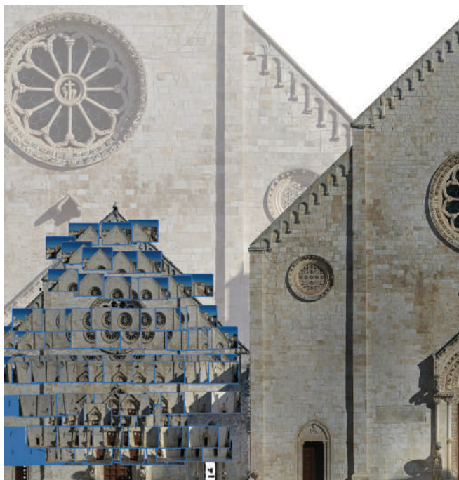
Figure 5. Extract of photogrammetry and dense cloud with location of main elevation photos.
