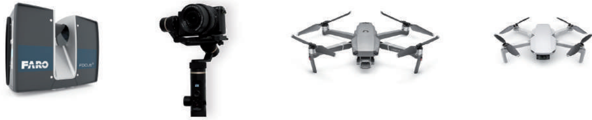
Figure 3. The Different types of instruments used by the Dada-Lab Research Laboratory during the acquisition campaign. From left: FARO CAM2 S150 terrestrial laser scanner, 3D-EYE, DJI Mavic 2 and Mavic Mini.
