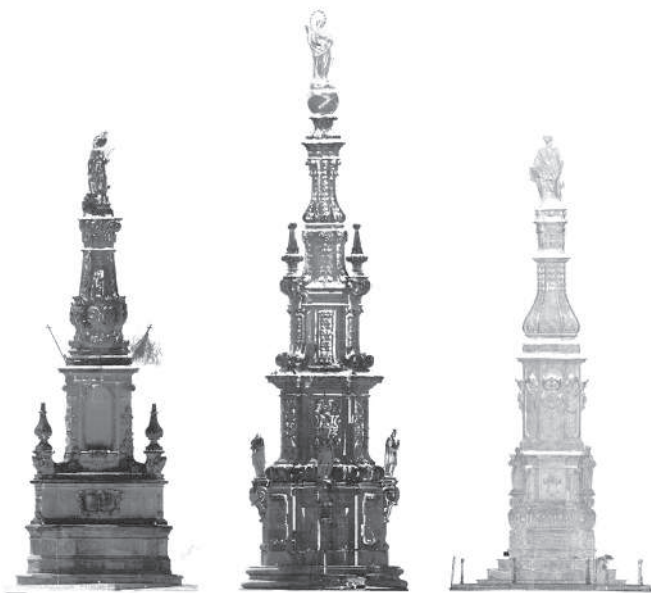
Figure 3. Areas without data in the orthographic views of the spiers's of Lequile, Nardò and Vernole points cloud.
