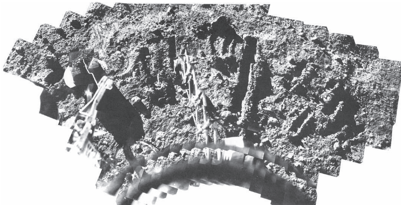
Figure 10. Surveyor 7: photographic mosaic of the sector dug by the mechanical arm.
