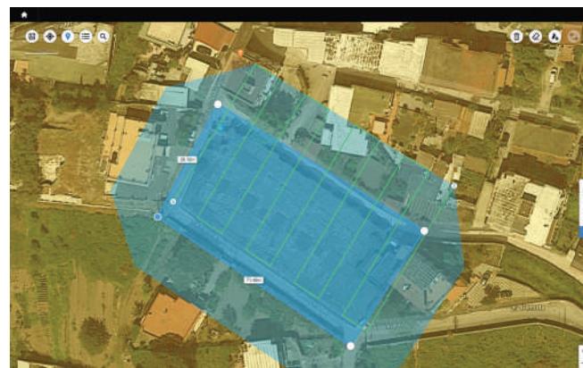
Figure 5. Oblique flight mission setup in DJI Terra software.
