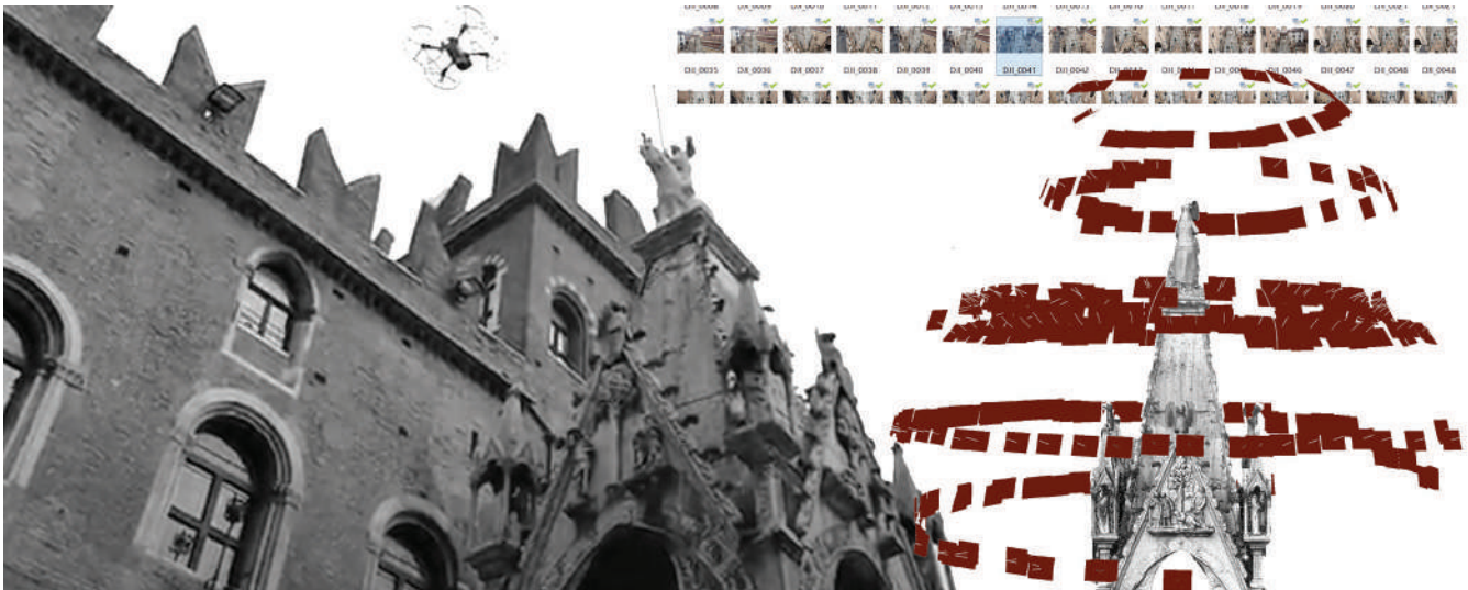
Figure 5. Drone acquisition methodology according to convergent axes of the upper portion of Ark of Mastino II.
