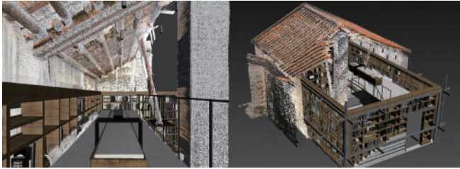
Figure 7. The point cloud model combined with the design model.
