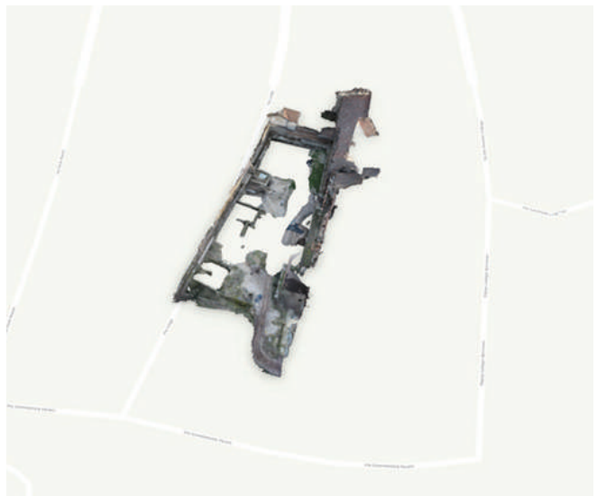
Figure 8. M(a) and RC(c) models overlapped and georeferenced in ArcGIS Pro.
