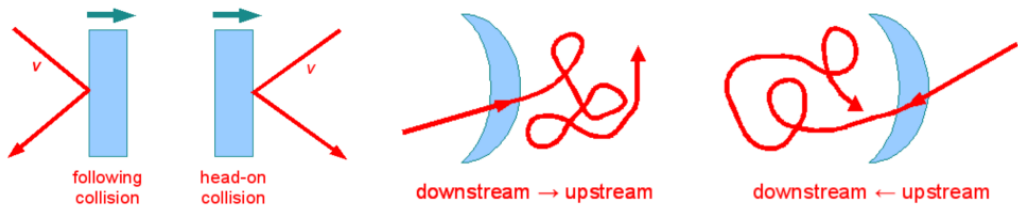
Figure 1.12: Schematic representation of Fermi acceleration mechanisms. On the left is the Fermi-II, resembling a ball bouncing elastically on walls. On the right is the Fermi-I, showing the motion of the shockwave front.
