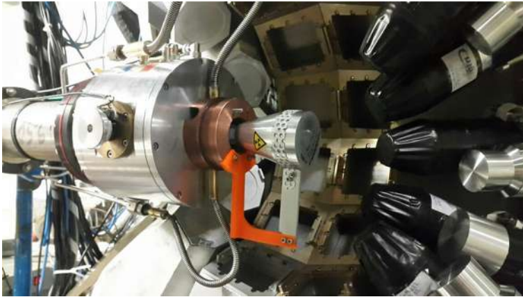
Fig. 47 The LICORNE neutron source coupled to the nu-Ball spectrometer [31] at the ALTO facility, IJC Lab. The sample in the center of the array is 71 g of ^{238}\text{U} metal turnings encapsulated in a thin aluminum case and is irradiated via the direction cone from LICORNE [369, 370]. The average target density is 0.7\text{ g/cm}^3 thus minimizes attenuation of low-energy \gamma rays
