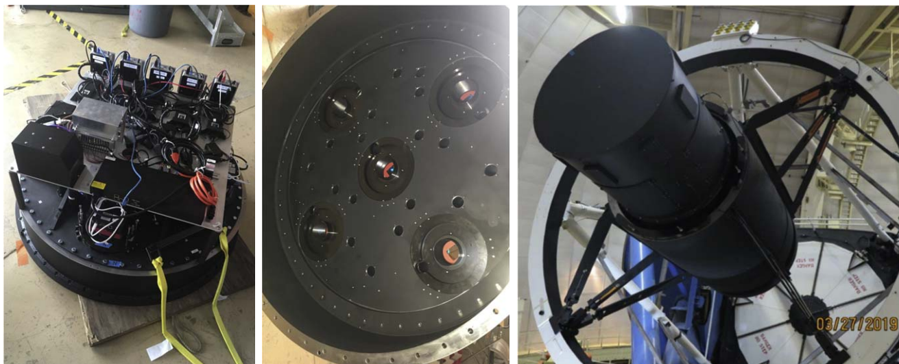
Figure 23. Three views of parts of the Commissioning Instrument (CI). (Left) Top view of the CI FPA. This side shows most of the electronics and faces away from the corrector. The electronics are mounted on a platform above the cameras and illuminated fiducials. (Middle) View of the CI that faces the corrector. The five larger apertures are for the five SBIG cameras, with one at the center of the FOV and the others near the periphery in the four cardinal directions. There are also 22 smaller apertures, each of which houses one of the illuminated fiducials. (Right) View of the CI after installation on the new corrector in late 2019 March.
