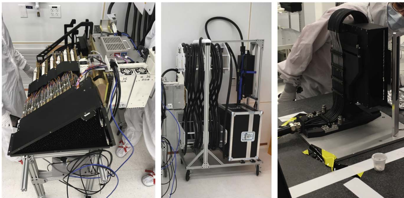
Figure 9. Photo of one of the ten DESI petal assemblies on 2019 February 21 in a clean room at the LBNL. The petal assembly includes the petal, fiber cable, and slithead. (Left) Petal with all 502 positioners, 12 fiducials, and the GFA unit, which will be aligned with the focal surface produced by the corrector. The black, triangular structure is a temporary, protective housing around these components. Behind this structure are the FIPOS electronics that drive the fiber positioners and fiducial LEDs, and wire and fiber guides. The petalbox electronics are to the right. (Middle) The \sim 50 m fiber cable that will extend from the petal in the focal plane system to a slithead in one of the 10 spectrographs. In this photo, the slithead is inside the protective case on the lower right on the cart. (Right) One of the DESI slitheads. The fiber cable attaches from the left in this photo. The pseudo-slit of fibers is pointed at an illumination system on the right.
