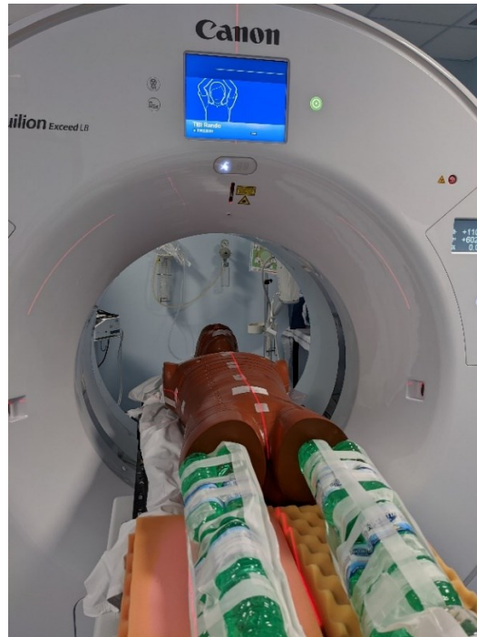
Figure 11. CT acquisition of Alderson Rando phantom with legs made of bottles of water in order to reach 180 cm height.
