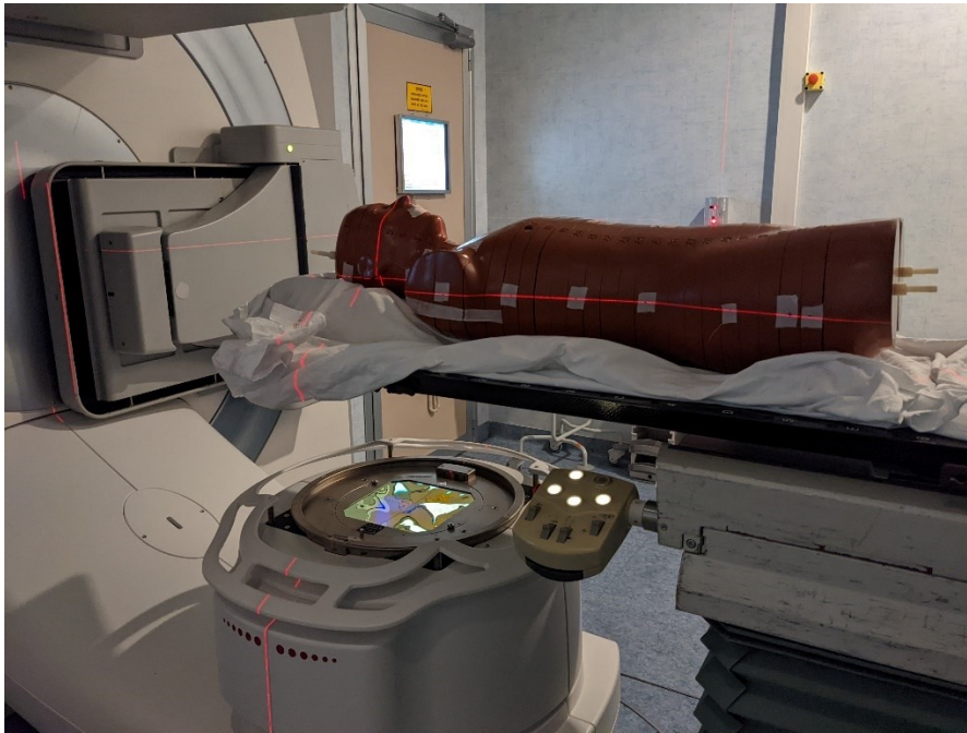
Figure 18. Alderson Rando positioning for VMAT-based TBI delivery.
