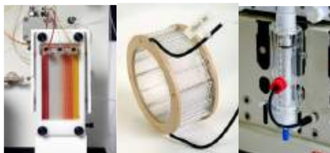
Figure 16. From left to right: a chip reactor, a coil reactor and a packed-bed reactor-
