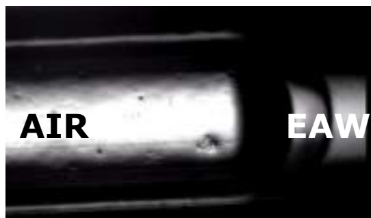
Figure 35. Disposition of a bubble of gas (AIR), the ethyl acetate (EA) and a buffer (W) segment inside the tubular microreactor.
