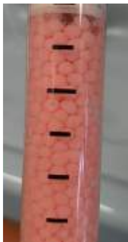
Figure 29. Packed bed reactor with R. rubra PVA/alginate and PVA beads.
