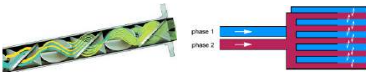
Figure 18. Static mixer (on the left). Multilamination-type micromixers (on the right): flow stream is divided in smaller streams increasing the contact interface between the solution enhancing diffusive mixing which takes place in short time thanks to the short diffusion path.
