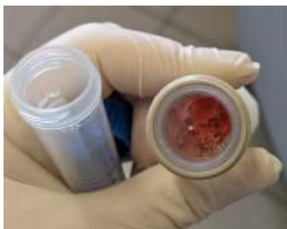
Figure 28. Destroyed alginate beads of R. Rubra by the excessive pressure inside the bioreactor.
