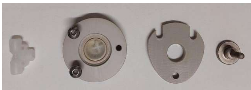
Figure 15. Photograph of a disassembled CSTR (fReactor) unit.
