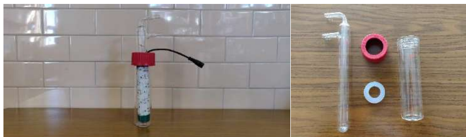
Figure 64. Photographs of the assembled and disassembled water-cooled photoreactor for cryogenic continuous flow operations
