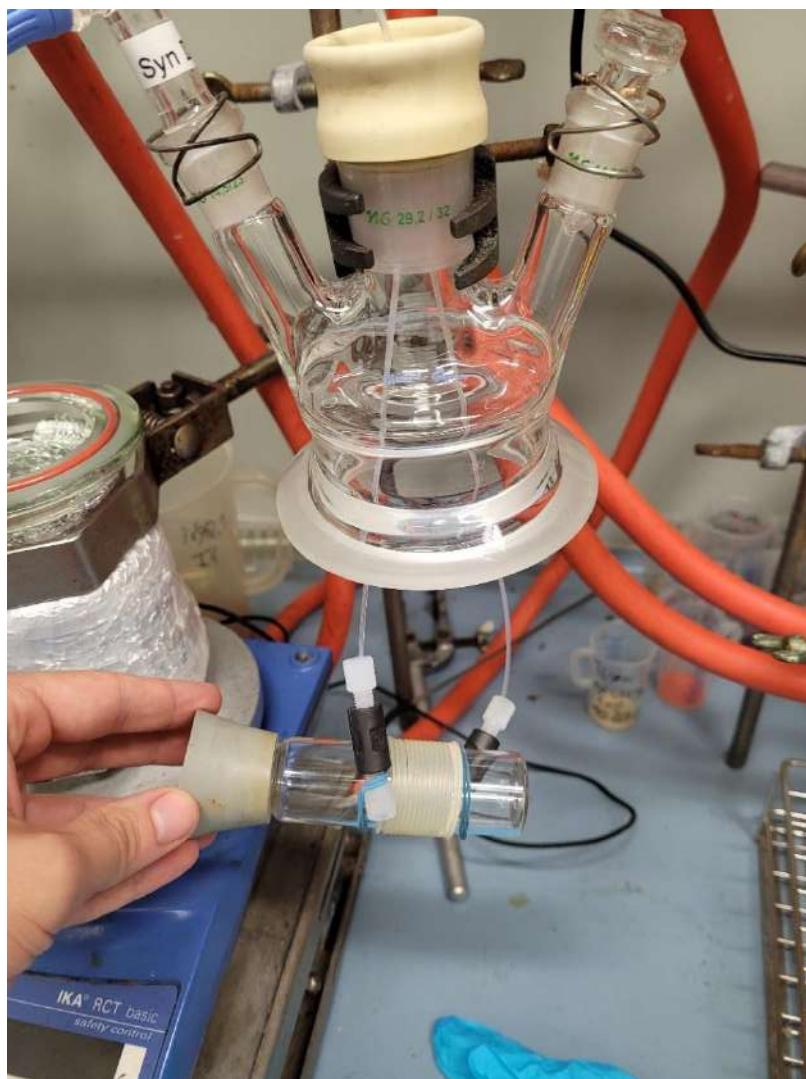
Figure 31. Photograph of the packed bed reactor (HPLC-tubing) filled with the solid supported 1 st generation MacMillan catalyst.
