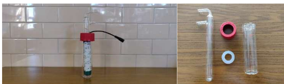
Figure 53. Photographs of the assembled and disassembled water-cooled photoreactor for cryogenic continuous flow operations
