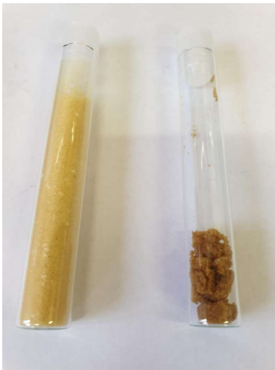
Figure 27. Photograph of the MR-1 st -Gen MacMillan (left) and TG-1 st -Gen MacMillan (right). Material color indicates absorption of violet-blue light.
