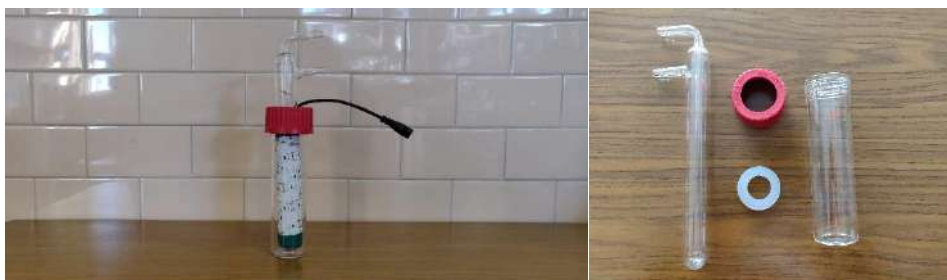
Figure 60: Photographs of the assembled and disassembled water-cooled photoreactor for cryogenic continuous flow operations
