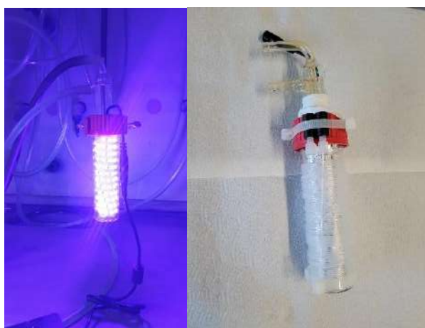
Figure 52: Photograph of the ignited watercooled high intensity LED photoreactor for cryogenic continuous flow operations. Photograph of the coil-reactor Perfluoroalkoxyalkane (PFA) HPLC-Tubing that is wrapped around the aforementioned photoreactor.
