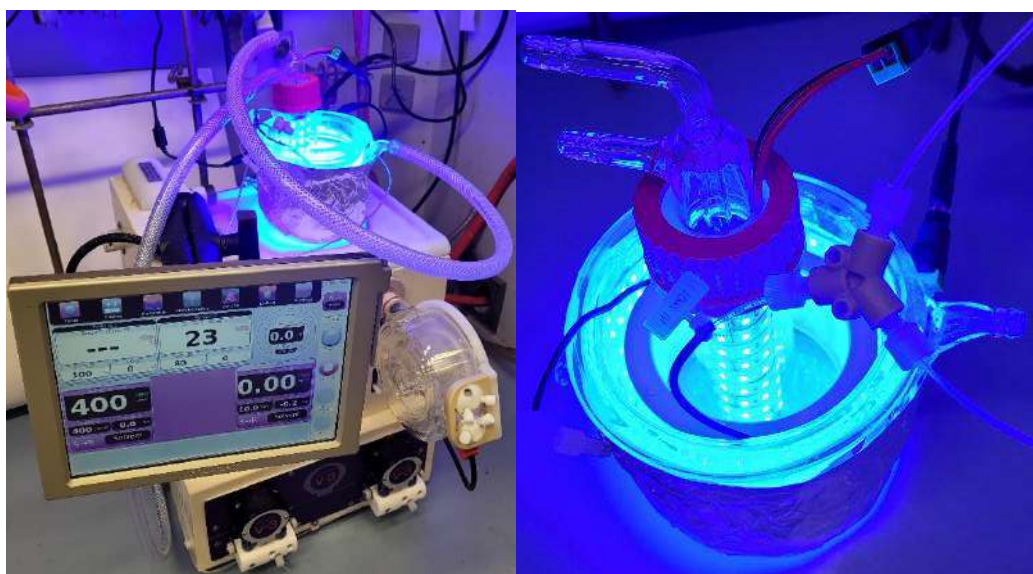
Figure 65. Assembly of the double walled glass photoreactor-couple with the central photoreactor on top of the VapourTec EasyScholar system.
