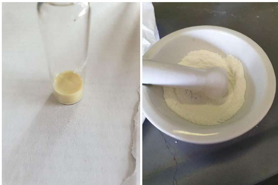
Figure 19. Photographs of the mesoporous copolymer just after the reaction is finished (left). Grinding of the polymer is required to get a fine material (right).
