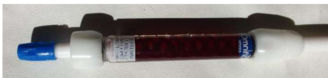
Figure 32. Photograph of the packed bed reactors that was build from an omnifit column, glass balls and MR-EY.
