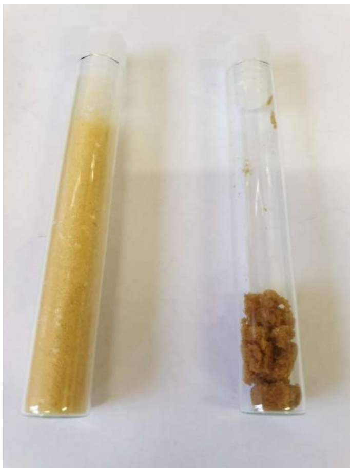
Figure 22. Photograph of the MR-1 st -Gen MacMillan (left) and TG-1 st -Gen MacMillan (right). Material color indicates absorption of violet-blue light.
