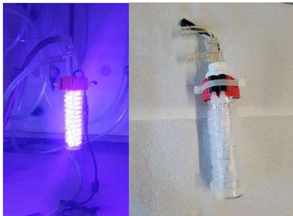
Figure 59: Photograph of the ignited watercooled high intensity LED photoreactor for cryogenic continuous flow operations. Photograph of the coil-reactor (12.33 m, 0.04 in ID Perfluoroalkoxyalkane (PFA) HPLC-Tubing that is wrapped around the aforementioned photoreactor.
