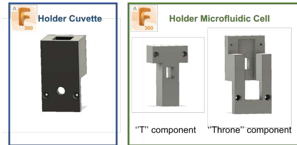
Figure 3.19: Aluminium holder components to host standard quartz cuvette (in blue box) and microfluidic cell (in green box) devised and designed with AutoDesk Fusion 360.
