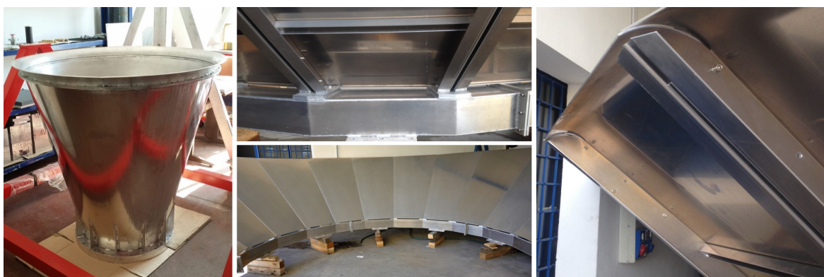
Figure 24. The FB during manufacturing (left) and details of the GS: base (top middle), inner panels (bottom middle) and flare (right).
