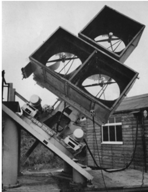
Fig. 2.2: Jelley's "light receiver" in 1961, Harwell (UK): three 1 m f/0.5 mirrors mounted equatorially for drift scans [60]. In following years the light collecting area would be increased using a cluster of small mirrors with a common focus.
