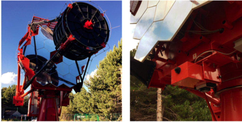
Fig. 3.22: Two pictures of the ancillary devices mounted on board the telescope ASTRI-Horn. The Pointing Monitoring Camera (PMC) is mounted inside the red cylinder on the back of the M2 support structure ( left ) and the auxiliary instrument UVSCOPE is installed below the primary mirror ( right ).
