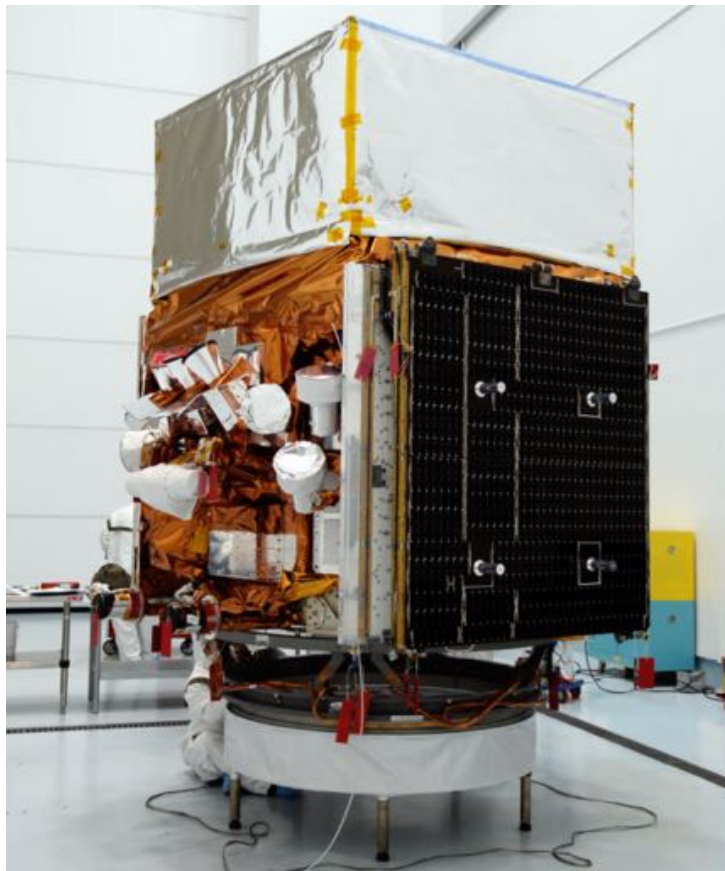
Fig. 1.9: The Fermi satellite before launch. The box on the top is the LAT instrument, composed of 4 \times 4 towers of silicon detectors to measure the direction of the incoming GR photons, with a calorimeter at the bottom measuring the energy of the electron/positron pairs. Credit: NASA/Kim Shiflett.
