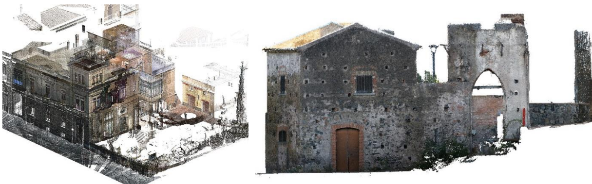
Fig: 1. On the left: view of the point cloud of villa Zingali - Tetto; On the right: view of the Noria's point cloud.
