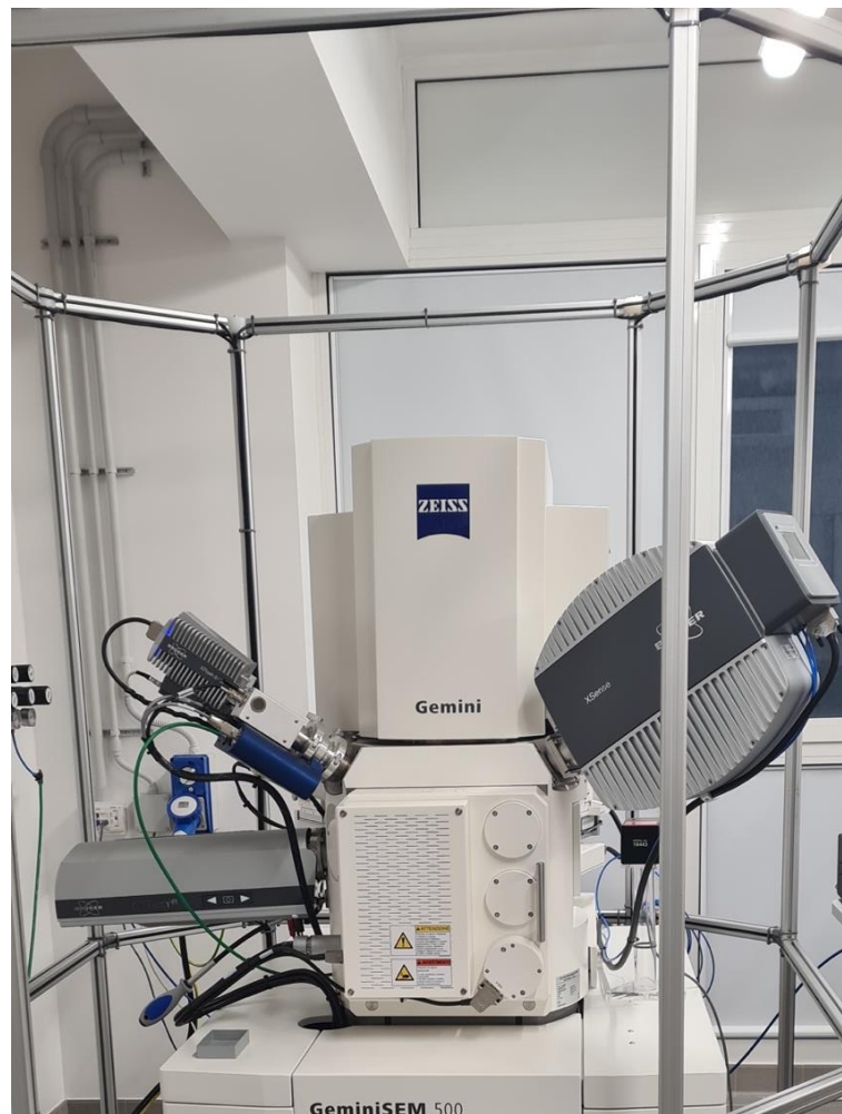
Figure 2-6 FEG-SEM Zeiss Gemini 500 at the Platform of Microscopy of the University of Milano-Bicocca.
