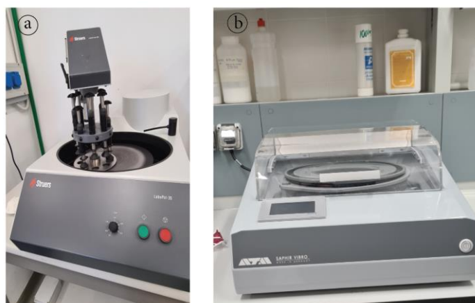
Figure 2-8 (a) Struers LaboPol-35 used for polishing samples with different diamond grain size paste and (b) Saphir Vibro used for chemical-mechanical polishing (CMP).
