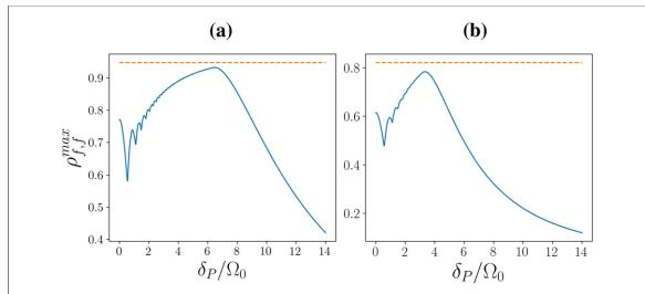
**Figure 8.** Maximum target-state population reached during the transfer performed using a protocol with  $\delta = 0$  and a constant value of  $\delta_P$  for the system in figure 2. The dashed horizontal line indicates the population of the target state achieved using protocol 1. In panel (a) [panel (b)] we have used  $\Omega_0 T = 40$  [ $\Omega_0 T = 20$ ].
