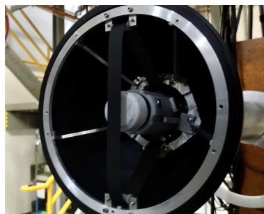
Figure 2.5: Zero Degree Scintillator detector mounted in the downstream hemisphere of the vacuum chamber. The detector is placed behind the tape where the beam is implanted.
