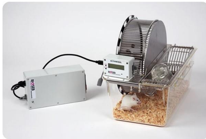
Figure 10 Activity wheel (BIO-ACTIVW-M – from Bioseb, in vivo research instruments).
