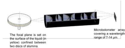
**Scheme 1:** Illustration of the infrared-relay lenses setup use to magnify the thermal image of the several hundred microns liquid gap.
