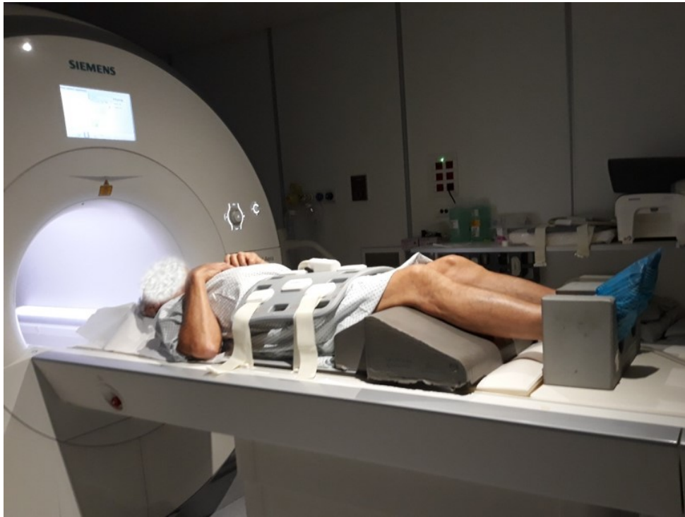
Fig. 7: Patient positioned on the 8 mm wooden bi-laminate rigid flat table, with fixation devices and 18-channel body RF coils, ready for MRI acquisition.
