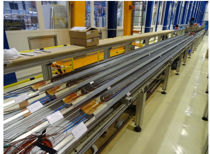
Figure 12. Four coils of MQXFB ready for assembly.
