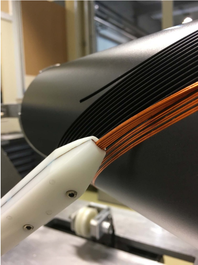
Figure 59. Tooling allowing to wind ten strands in one go.
