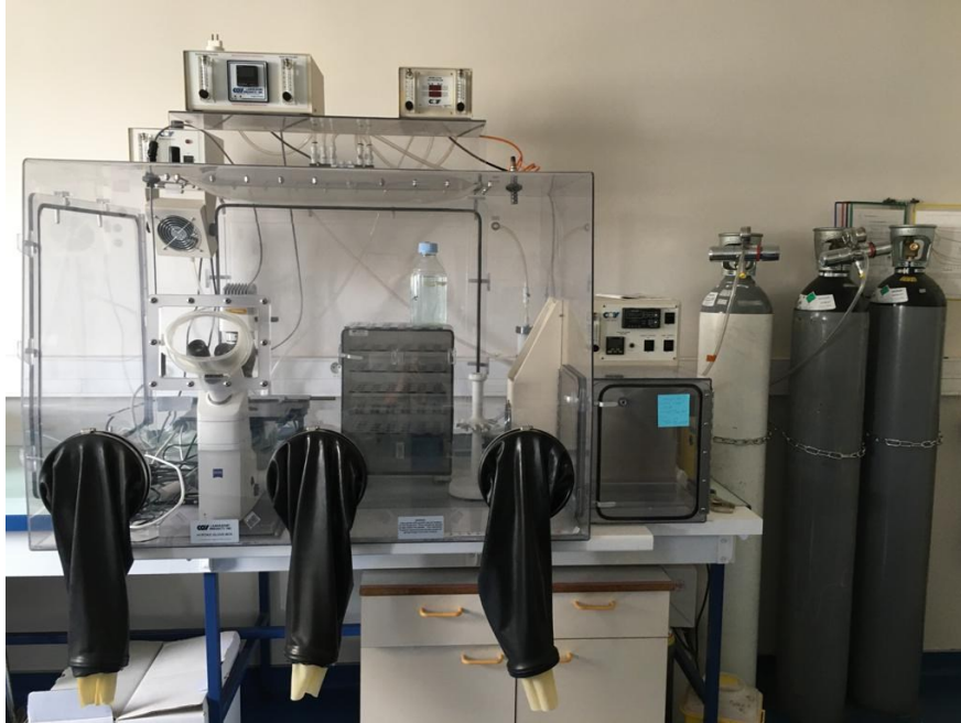
Figure 5: Hypoxic chamber, a way to test the effects of hypoxia in cell models, Creteil, Université Paris Est
