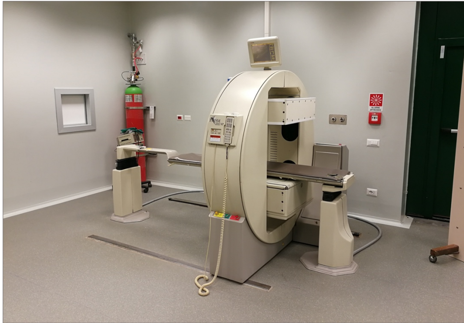
Figure 1.5 The SPECT gantry with a single head gamma camera used in the UNIMI Veterinary Teaching Hospital, (Lodi).
