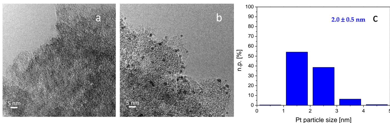
**Figure 5.** Representative TEM images collected on Pt-Mo(NH<sub>4</sub>)\_fresh (a) and Pt-Mo(NH<sub>4</sub>)\_400N (b). Particle size distribution of the sample treated at 400 °C in N<sub>2</sub> (c). Instrumental magnification: 100000X and 250000X, respectively.
