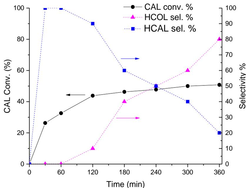
**Figure 2.** CAL hydrogenation reaction profile vs. time. CAL conversion % (solid line, left Y axis) along with HCAL and HCOL selectivity % (dashed lines, right Y axis) over Pt-Mo(NH<sub>4</sub>)<sub>400N</sub>.
