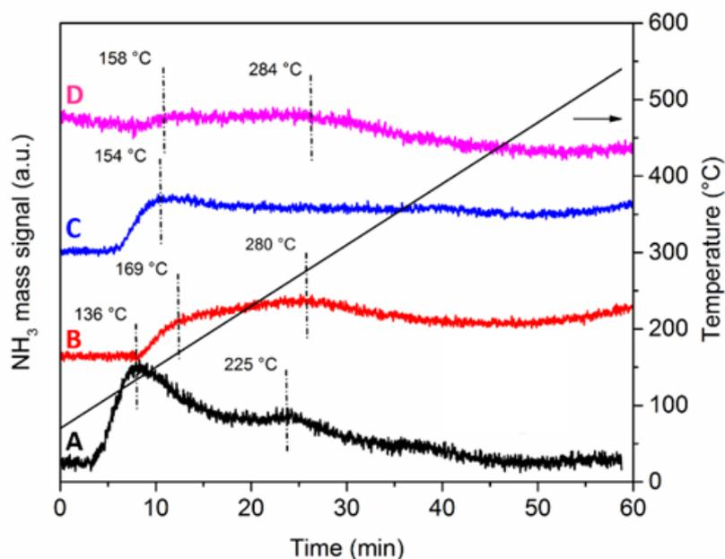
**Figure 6.** NH<sub>3</sub>-TPD profiles of the Pt-Mo(NH<sub>4</sub>)<sub>fresh</sub> (A) and Pt-Mo(NH<sub>4</sub>)<sub>400N</sub> (B) samples, and of the Pt-Mo(Na)<sub>fresh</sub> (C) and Pt-Mo(Na)<sub>400N</sub> (D) samples.
