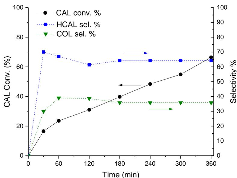
**Figure 3.** CAL hydrogenation reaction profile vs. time. CAL conversion % (solid line, left Y axis) along with HCAL and COL selectivity % (dashed lines, right Y axis) over Pt-Mo(Na)<sub>400N</sub>.
