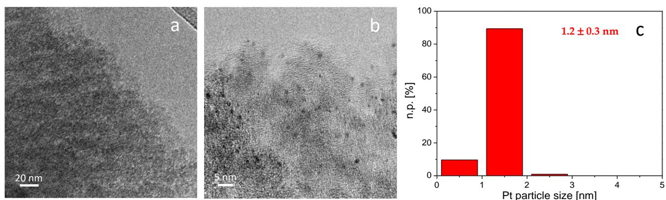
**Figure 4.** Representative TEM images of Pt-Mo(Na)\_fresh (a) and Pt-Mo(Na)\_400N (b). Pt particle size distribution of the sample treated at 400 °C in N<sub>2</sub>(c). Instrumental magnification: 100000X and 250000X, respectively.
