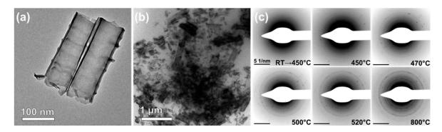
**Figure 1.** *In situ* selected area electron diffraction (SAED) heating experiment: (a) Representative (TiO2 amorphous nanotubes) TANs at room temperature RT; (b) The several micron-sized aggregate of TiO<sub>2</sub> TANs chosen for the *in situ* heating; (c) SAED patterns of the aggregate reported in panel (b), recorded at different temperatures during the *in situ* heating experiment.
