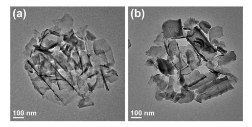
**Figure 2.** Low magnification transmission electron microscopy (TEM) images of micron-sized TANs: (a,b) Small aggregates of TANs recorded at RT and used for the *in situ* high resolution transmission electron microscopy (HRTEM) heating experiment.
