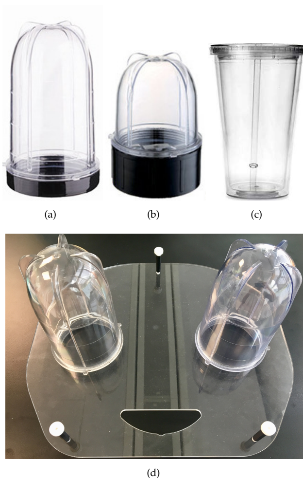
Figure 5.1: (a-b-c) Jars of different sizes to mimic the breast shape. (d) Jars and support base assembled to build the shell of BREATH.
