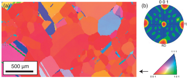
FIG. 2. (Color online) (a) Electron back scattering diffraction map acquired on a graphene grown on Cu foil sample. (b) Orientation distribution of the image reported in (a). The dominant crystalline orientation is (001).
