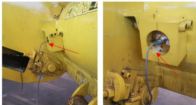
Figure 1. Positioning of the sensor behind the loading drum of the conveyor arm of the wagon. The sensor is indicated with a red arrow. MS was flanged with a 5-cm thick holder metal ring to avoid electrical interference effects.
