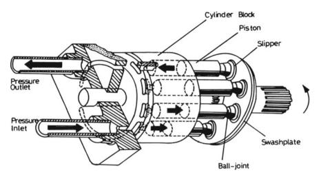
Fig. 14.1 Hydraulic piston pump
