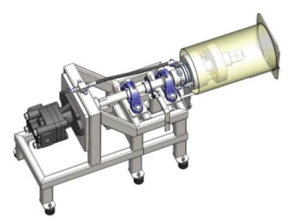
Fig. 14.3 Slipper test bench
