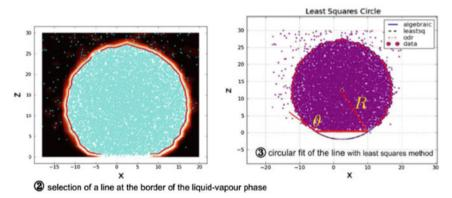
Fig. 14.4 Summary of the procedure adopted to extract the contact angle from MD results
