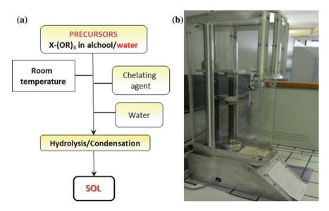
Fig. 14.2 a Sol-gel synthesis methodology; b dip coater
