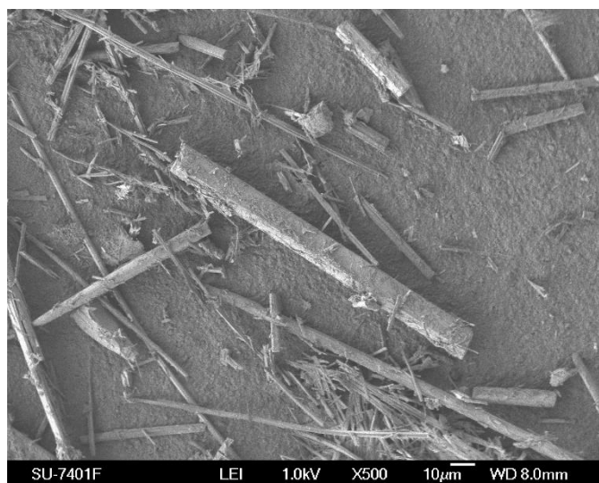
Figure S27. SEM micrograph of \text{Bi(OH)(H}_2\text{BPT)}_2(\text{H}_2\text{O})_2 \cdot \text{H}_2\text{O} ( 3 ), showing large bladed crystals together with small amounts of 2 .
