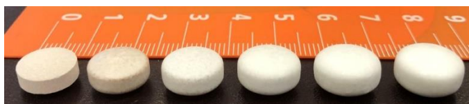
Figure 1. Photographs of uncoated cores and HPMC-coated systems having increasing coating level (ruler scale in cm).
