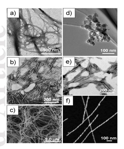
**Figure 2.** TEM images of a) MFC and b) CNCs; SEM micrographs of c) BC; d) SNCs (reproduced with permission from Elsevier Ltd [Wang *et al.*, 2010]); e) chitin nanocrystals (reproduced with permission from Elsevier Ltd [Wang *et al.*, 2012]); f) AFM image of amyloid fibrils with twisted ribbon morphology (reproduced with permission from Elsevier Ltd [Adamcik and Mezzenga, 2012]).
