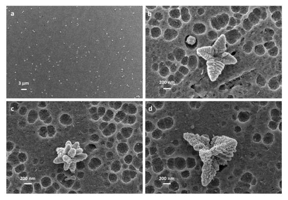
**Figure 3.** FE-SEM observations of CEL2 + pad (1 mg/mL) + Ag. (a) Low magnification overview of surface; (b–d) Ag precipitates as dendrimeric nanoflowers and holes on the glass surface due to reaction in the functionalization media (higher magnification).
