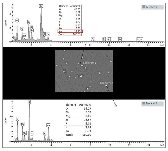
Figure 4. EDS analyses on CEL2 + pad (1 mg/mL) + Ag.
