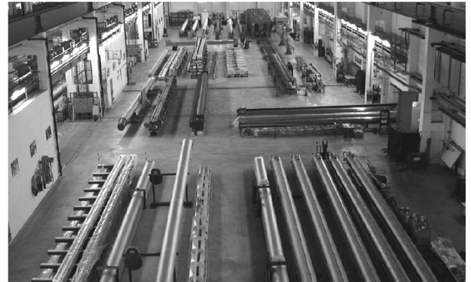
Fig. 1. LHC main dipole cold mass manufacturing at one of the 3 cold mass assemblers.
