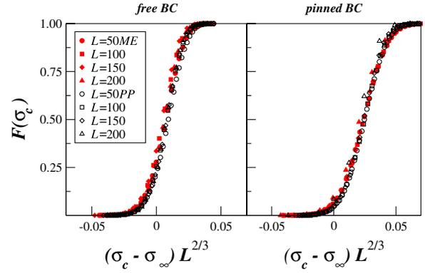
FIG. 2 (color online). Cumulative distributions of yield stress for free and pinned boundary conditions for ME and PP. The distributions can all be collapsed with the same exponent, related to  $\theta = 1/3$ .
