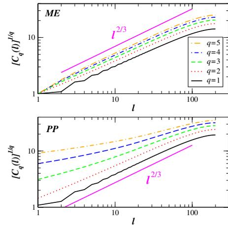
FIG. 3 (color online). Height-height correlation function of order  $q = 1$  to  $q = 5$  for ME and PP problems in a system of size  $L = 200$ . Multiscaling of the surface fluctuations for PP is clearly observed.
