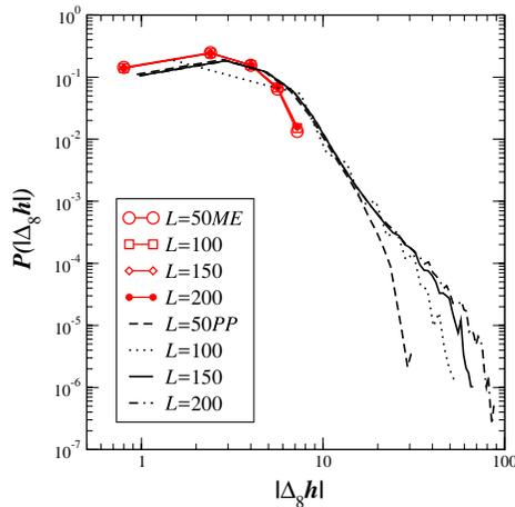
FIG. 4 (color online). Distribution of height differences at a fixed distance  $\ell = 8$  in PP and ME for different system sizes. For PP the tail of the distribution grows with system size, while it remains constant for ME surfaces.
