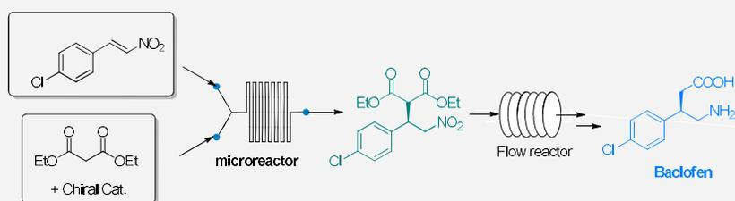
The potential of this flow chemistry approach was demonstrated by the successful synthesis of an advanced intermediate for the preparation of the GABA<sub>B</sub> receptor agonist Baclofen and other Active Pharmaceutical Ingredients (APIs) such as (*S*)-Pregabalin and (*S*)-Warfarin.
