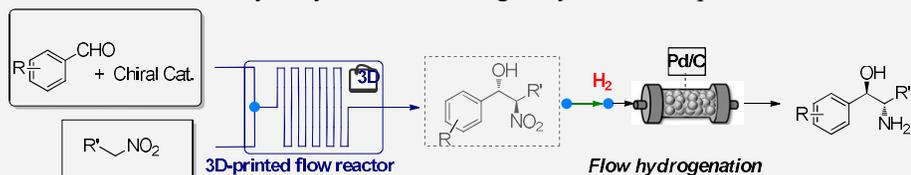
Norephedrine, Metamaminol and Methoxamine have been prepared through a two-steps sequence, involving a stereoselective Henry reaction promoted by a chiral copper catalyst, performed into 1 mL 3D-printed flow reactors made of different materials (PLA, HIPS, NYLON) and a continuous flow hydrogenation.<sup>3</sup>
