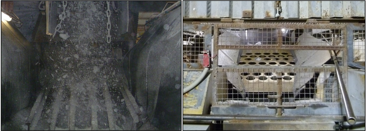
Figure 3.15 Vibrating screen, on the left the original version, on the right the modified one.
