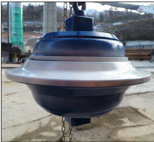
Figure 2.9 Single disc cutter.
