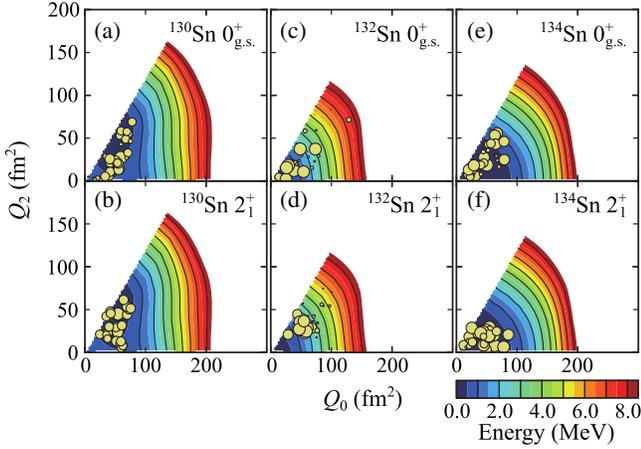
FIG. 4.  $T$ -plots of the  $0_{g.s.}^+$  (a,c,e) and  $2_1^+$  states (b,d,f) of  $^{130}\text{Sn}$  (a,b),  $^{132}\text{Sn}$  (c,d), and  $^{134}\text{Sn}$  (e,f) show a pronounced potential-energy minimum for the spherical doubly magic configuration. Circles on the PES represent shape dynamics of MCSM basis vectors. See text for details and discussion.
