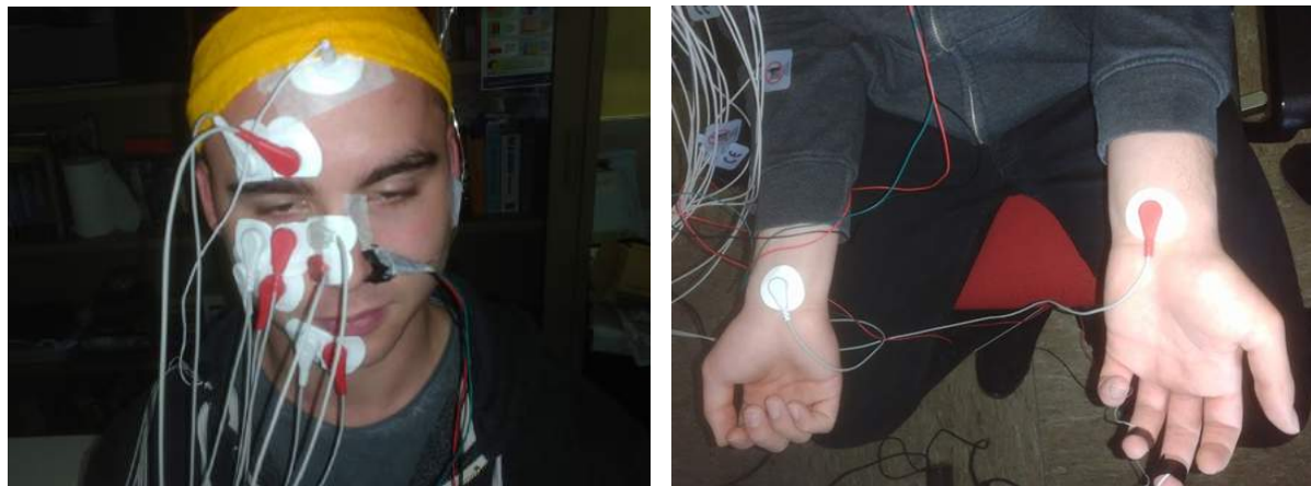
(A) Electrodes used to acquire facial EMG
