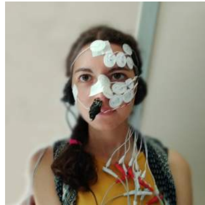
(B) Electrodes placement to acquire the facial EMGs, and respiration sensor placed under the participant's nose
