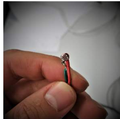
(D) Photoresistor used to collect the light on the VR headset lens
