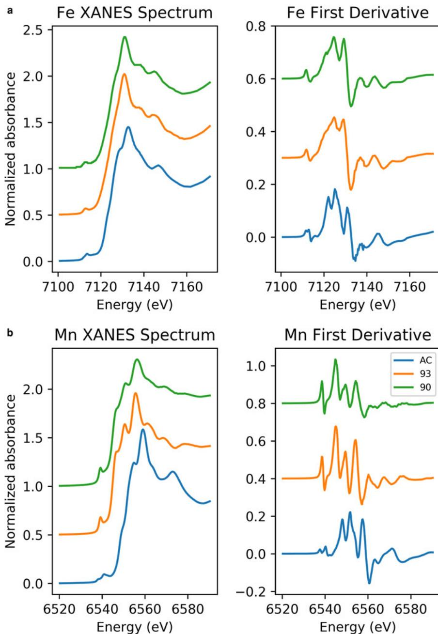
FIG. 2. (a) Fe *K*-edge XANES spectra of jacobsite spinel synthesized with: 93%, 90% CO<sub>2</sub> and no gas flow. (b) Mn *K*-edge XANES spectra of jacobsite spinel synthesized with: 93% CO<sub>2</sub>, 90% CO<sub>2</sub> and no gas flow.
