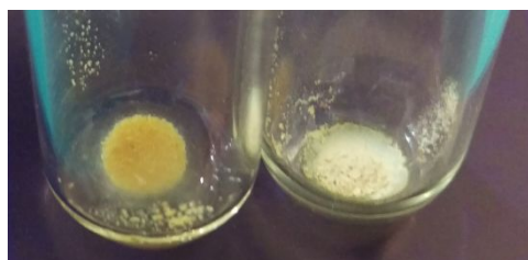
Figure S5. Visual detection of iodine release for 15 mg a) 1-I 2 and b) KEZXEU-I 2 immersed in 2 ml EtOH. c) Absorbance-time profile for the release of iodine from 15 mg 1-I 2 (blue) and KEZXEU-I 2 (orange) immersed in 3 ml EtOH. d) Solid materials of compounds 1 (left) and KEZXEU (right) recovered from EtOH solutions after iodine release.
