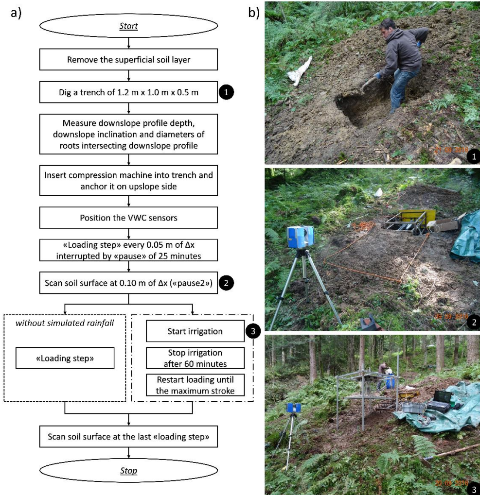
Figure 6.4. a) Flowchart of the experimental procedure; and b) photographs at different stages of an experiment.
