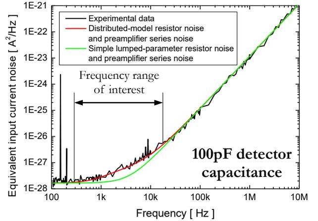
Fig. 3. Input referred current noise of a charge-sensitive preamplifier with the integrated  $100\text{M}\Omega$  resistor as feedback. For a charge-sensitive preamplifier the noise corner frequency goes like the inverse of the total input capacitance. If either the series noise or the input capacitance are high, the noise corner frequency can become so low that the contribution of the  $f$ -like noise component from the resistance with distributed capacitance can be considered negligible.
