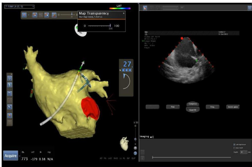
Figure 16B: Screen shot of the CARTO (Biosense Webster, Inc., Diamond Bar, Calif.) electroanatomical mapping system. On the right, in the ICE 2-D image, the green colored electronic representation of the catheter tip in left atrial chamber shows good contact to endocardial tissue. In the left panel high contact force confirmed good catheter tip-tissue contact
