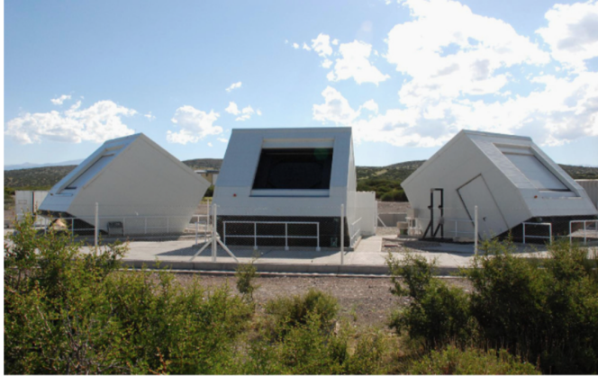
Figure 3.15: Picture of the three HEAT telescopes in tilted mode. The container for DAQ, slow control, and calibration hardware is behind the enclosure of the second telescope.
