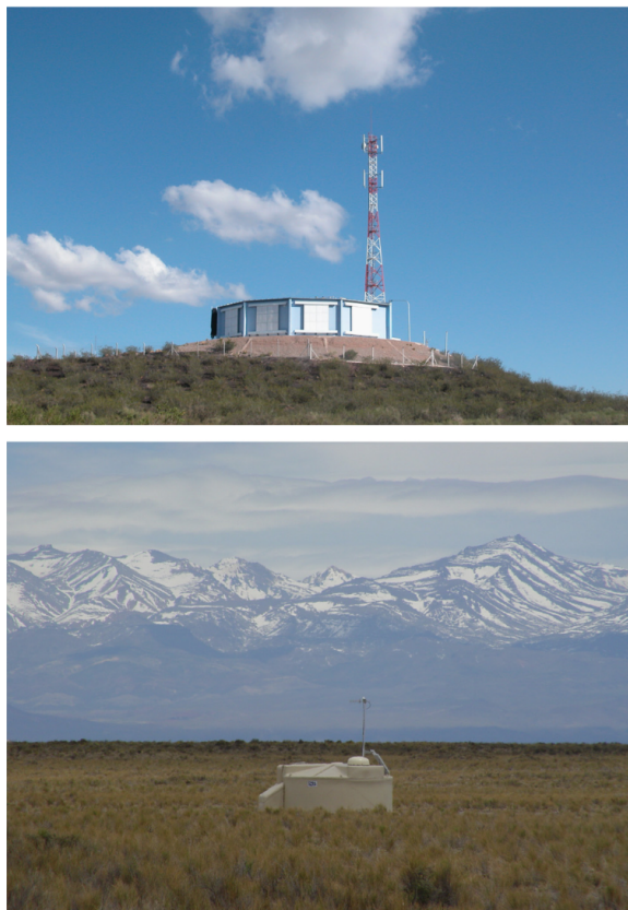
Figure 3.2: The fluorescence detector enclosure Los Leones (top panel) and a surface detector station (bottom panel).
