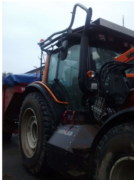
Figure 3. Valtra N101 tractor with the implemented system to collect exhaust gases for the gases analyser.
