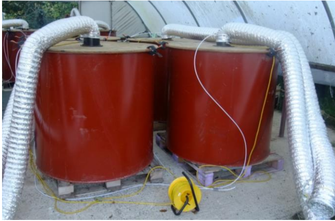
Figure 1. Pilot scale slurry storage tanks with specially adapted lids for gaseous emission measurements
