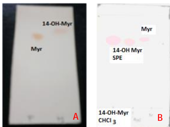
Figure 19. A) TLC of standard Myr after 1 hour reaction \text{NaBH}_4 under the condition described above. B) TLC of the product found in the chloroform extract before (left spot) and after SPE purification (central spot).
