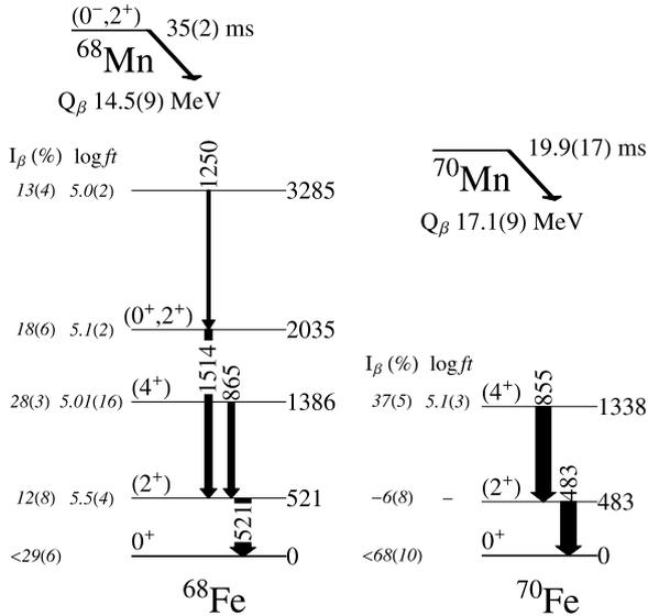
**Fig. 3.** Partial level schemes following the  $\beta$  decays  $^{68}\text{Mn} \rightarrow ^{68}\text{Fe}$  (left) and  $^{70}\text{Mn} \rightarrow ^{70}\text{Fe}$  (right).  $Q_\beta$  values are taken from Ref. [40].
