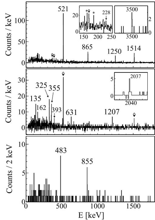
**Fig. 2.**  $\beta$ -delayed  $\gamma$ -decay spectra following the decays  $^{68}\text{Mn} \rightarrow ^{68}\text{Fe}$  (upper panel),  $^{69}\text{Mn} \rightarrow ^{69}\text{Fe}$  (middle panel) and  $^{70}\text{Mn} \rightarrow ^{70}\text{Fe}$  (bottom panel). Transitions belonging to  $^{68,69,70}\text{Fe}$  are labelled, while transitions populating the  $\beta$ -n channel are indicated by diamonds. The asterisks indicate transitions depopulating states in the grand-daughter nucleus.
