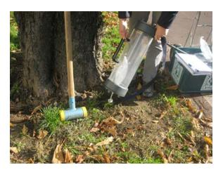
**Fig. 4.** The automatic pump employed in the field to put directly soil air in Nalophan bags.
