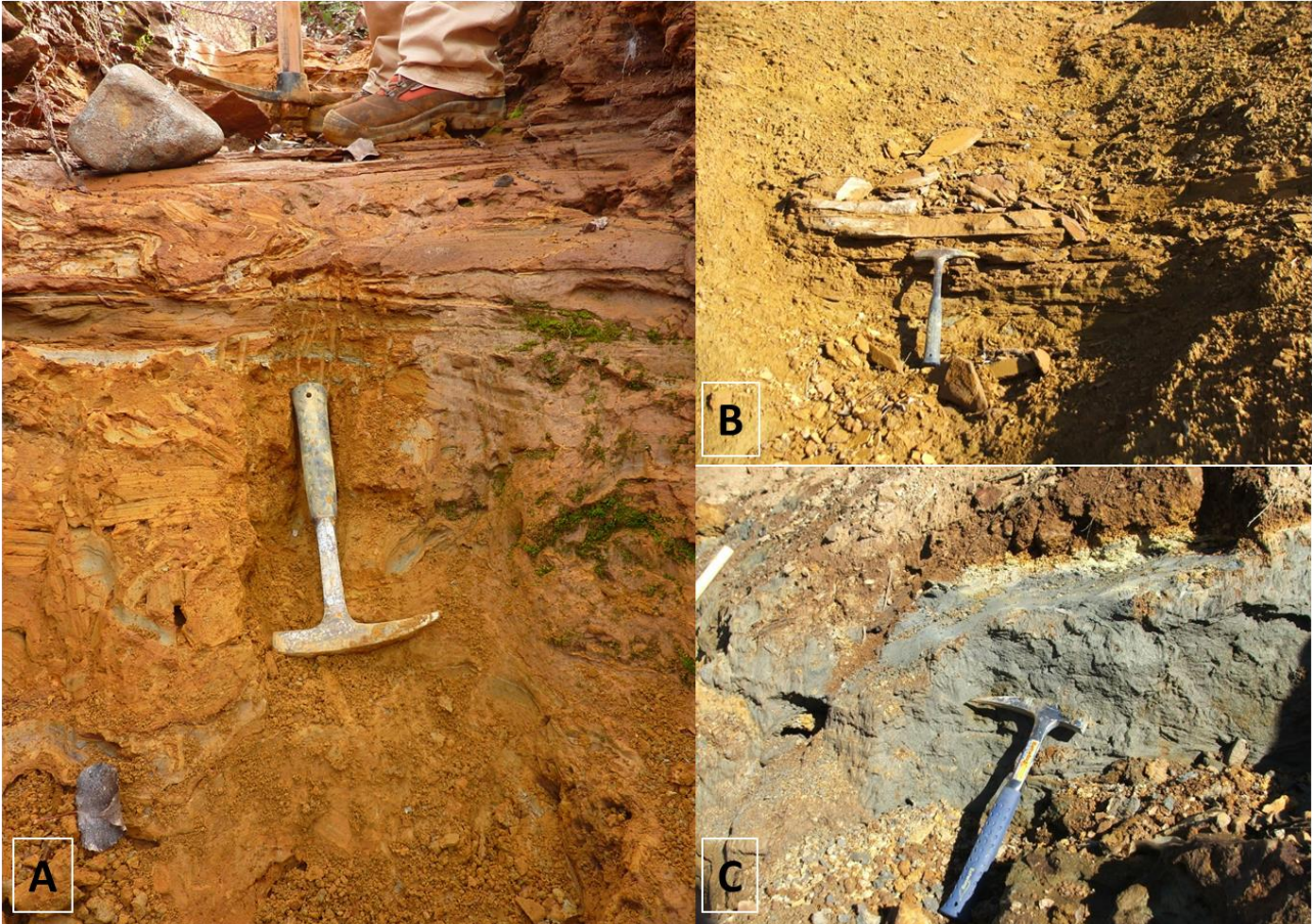
FIGURE 9 TAILING GEOMETRIES OBSERVED IN THE R2 DUMP A) FINELY LAYERED TAILINGS UNDERNEATH THE BACKFILL COVER B) LAYERS OF LS TAILING (SEE TEXT) C) HS TAILING (SEE TEXT) HORIZON
